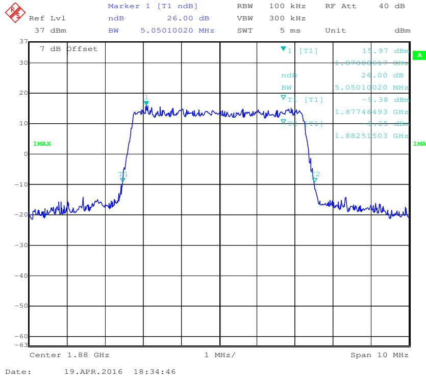
**16-QAM (5.0 MHz) - 99% Occupied Bandwidth, Middle channel**
