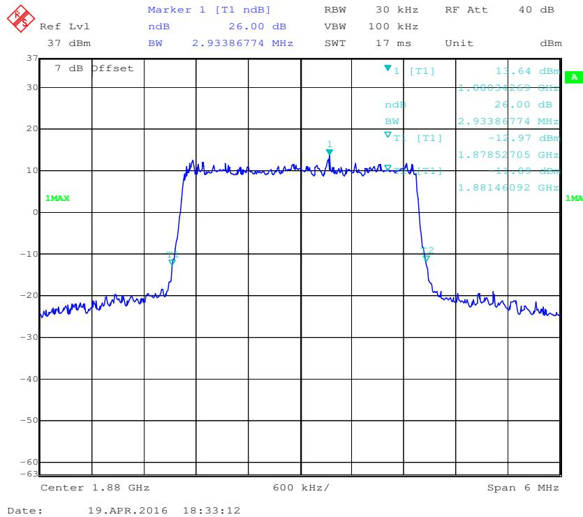
**QPSK (5.0 MHz) - 99% Occupied Bandwidth, Middle channel**
