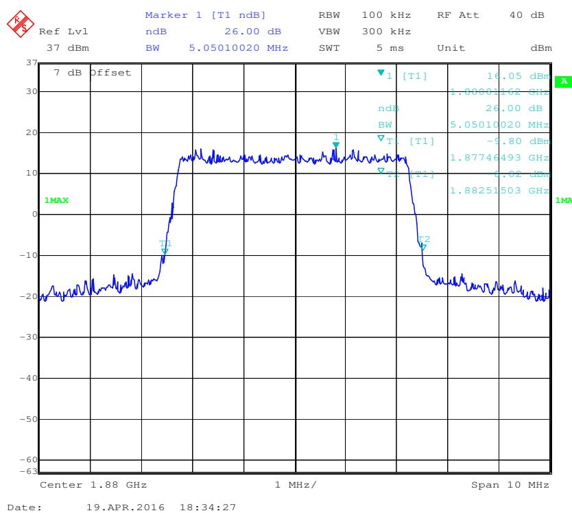
**QPSK (10.0 MHz) - 99% Occupied Bandwidth, Middle channel**
