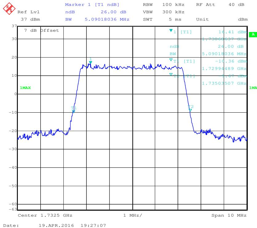
**QPSK (10.0 MHz) - 99% Occupied Bandwidth, Middle channel**
