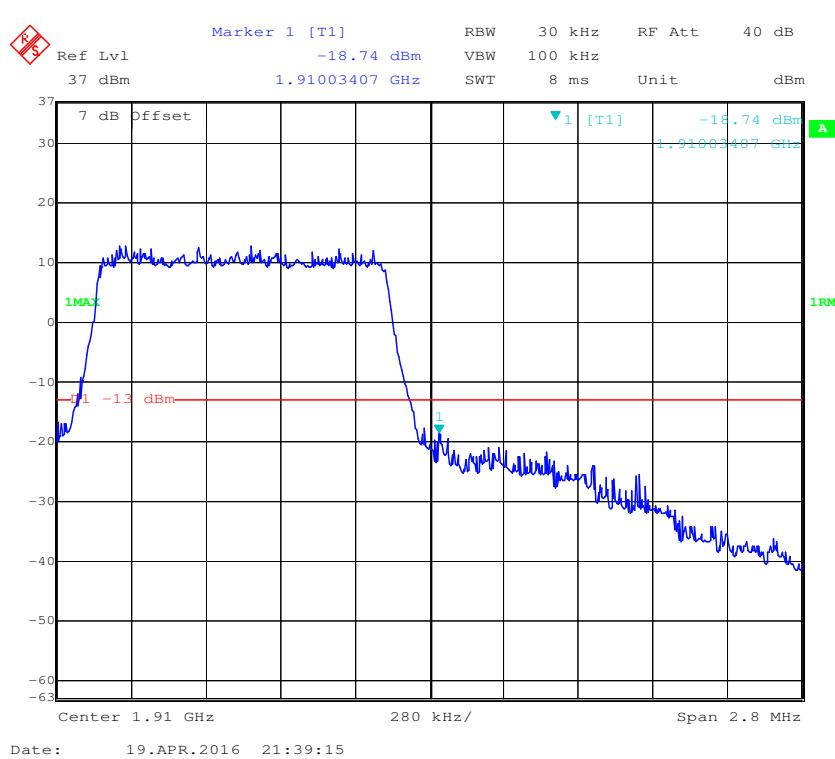
**16-QAM (1.4 MHz, FULL RB) - Left Band Edge**
