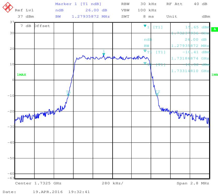
**16-QAM (1.4 MHz) - 99% Occupied Bandwidth Middle channel**
