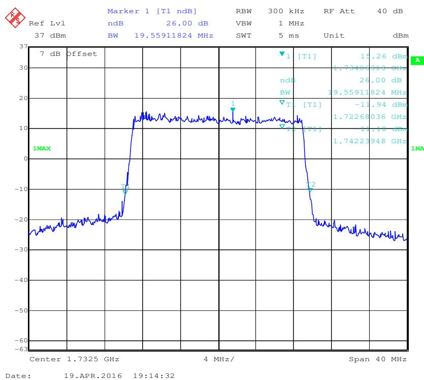
**16-QAM (20.0 MHz) - 99% Occupied Bandwidth, Middle channel**
