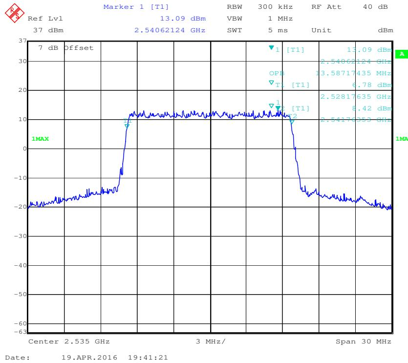
**16-QAM (15.0 MHz) - 26 dB Bandwidth, Middle channel**
