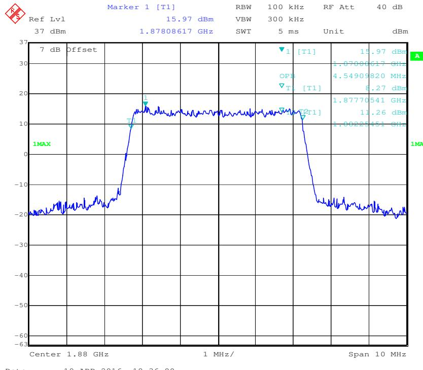
**16-QAM (5.0 MHz) - 26 dB Bandwidth, Middle channel**
