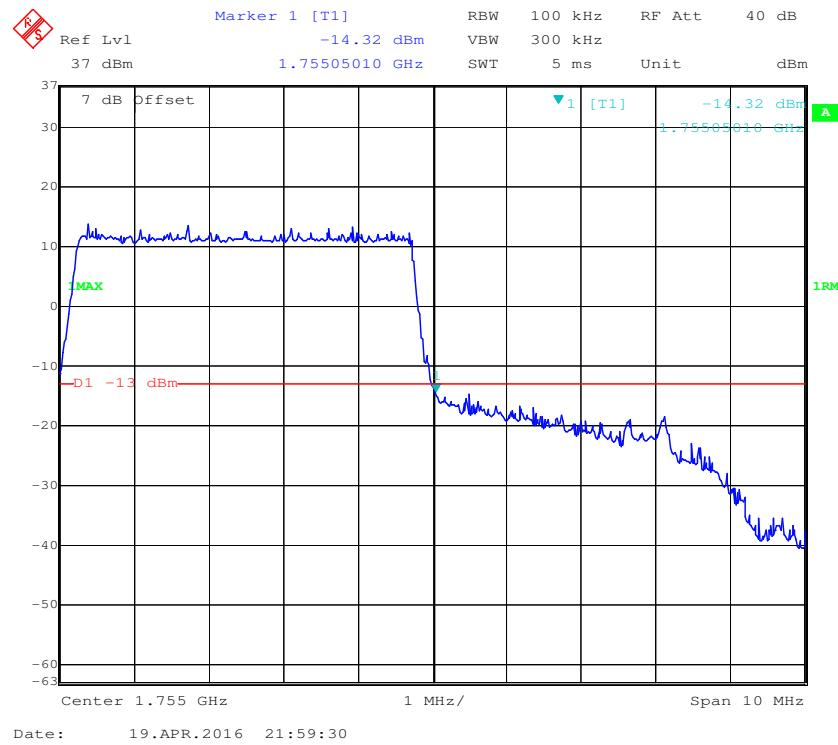
**16-QAM (5.0 MHz, FULL RB) - Left Band Edge**
