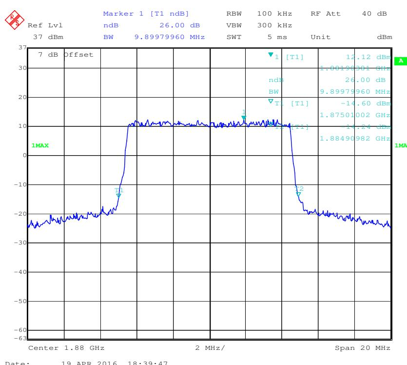
**16-QAM (10.0 MHz) - 99% Occupied Bandwidth, Middle channel**
