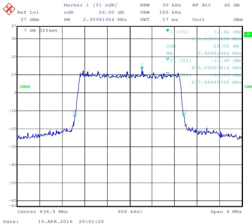
**16-QAM (3.0 MHz) - 99% Occupied Bandwidth, Middle channel**
