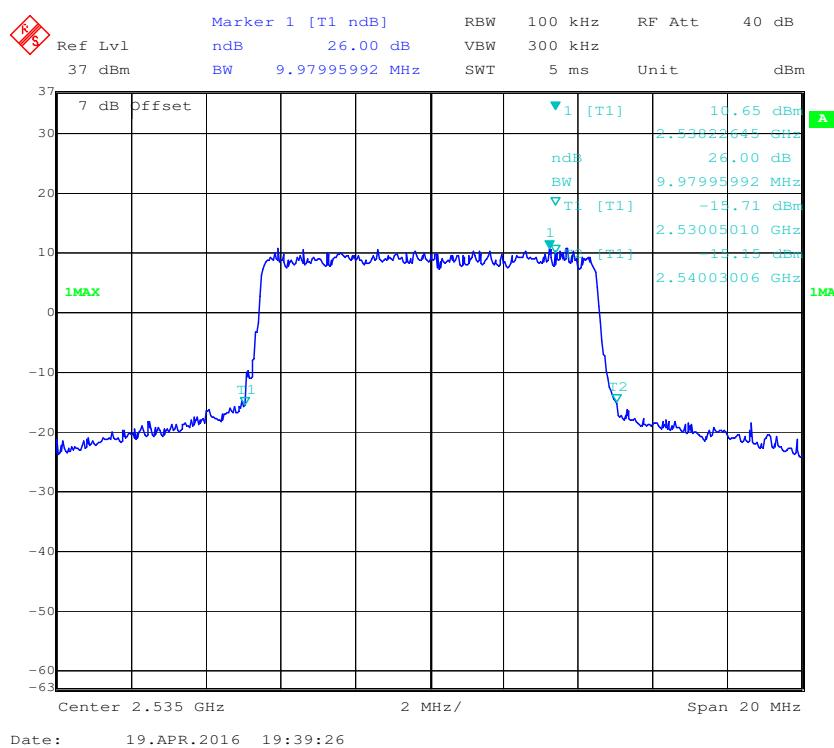
**QPSK (15.0 MHz) - 99% Occupied Bandwidth, Middle channel**
