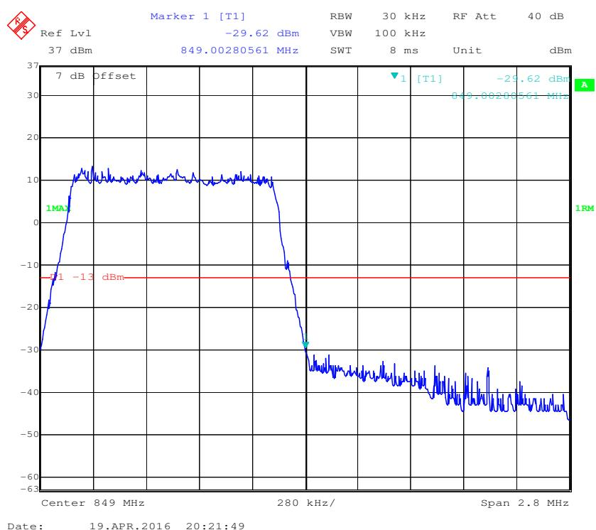
**16-QAM (1.4 MHz, FULL RB) - Left Band Edge**
