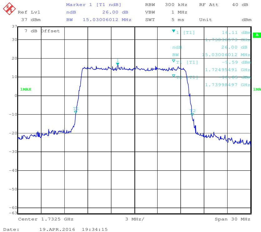
**QPSK (20.0 MHz) - 99% Occupied Bandwidth, Middle channel**
