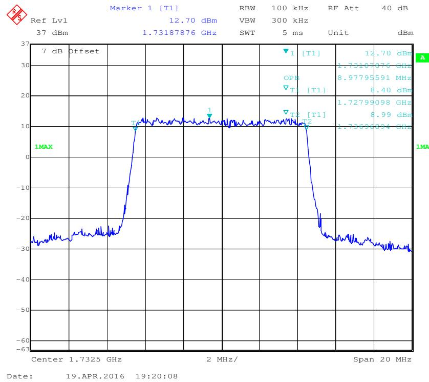
**16-QAM (10.0 MHz) - 26 dB Bandwidth, Middle channel**
