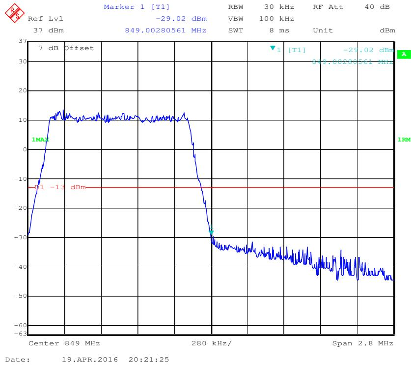
**QPSK (3.0 MHz, FULL RB) - Left Band Edge**
