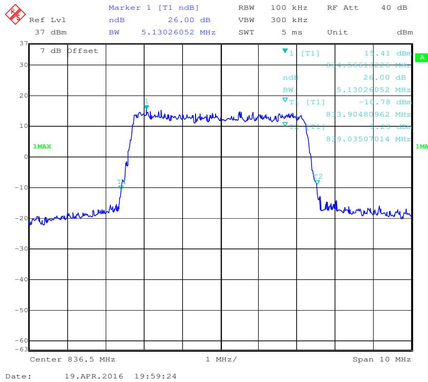
**QPSK (10.0 MHz) - 99% Occupied Bandwidth, Middle channel**
