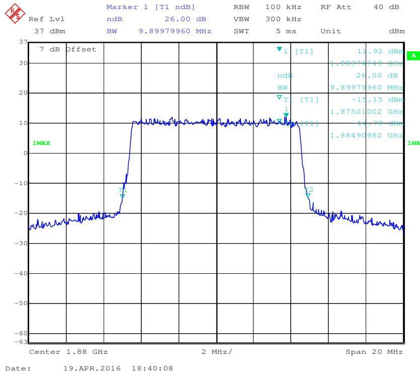
**QPSK (15.0 MHz) - 99% Occupied Bandwidth, Middle channel**
