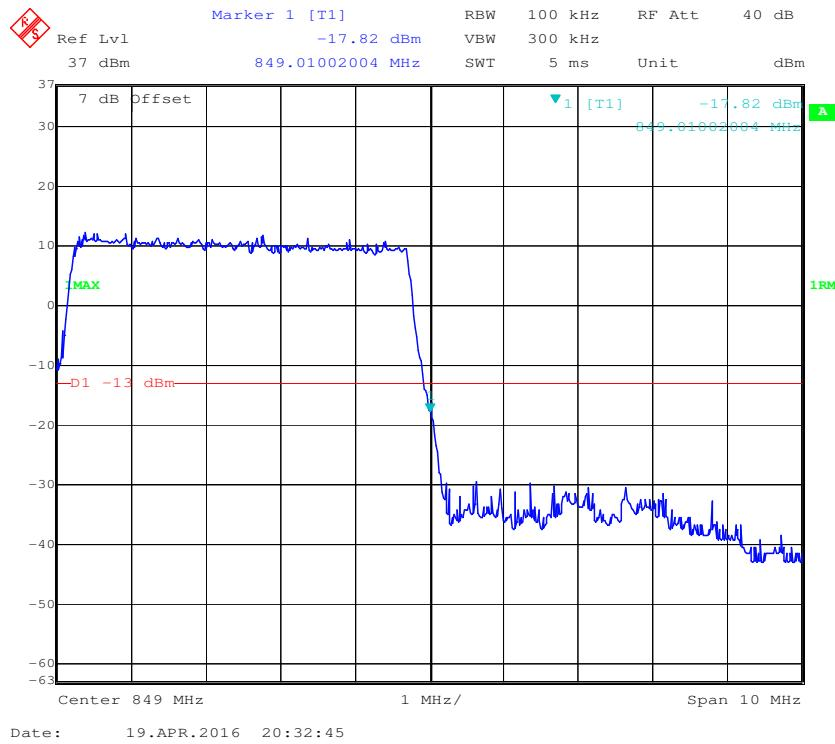
**16-QAM (5.0 MHz, FULL RB) - Left Band Edge**
