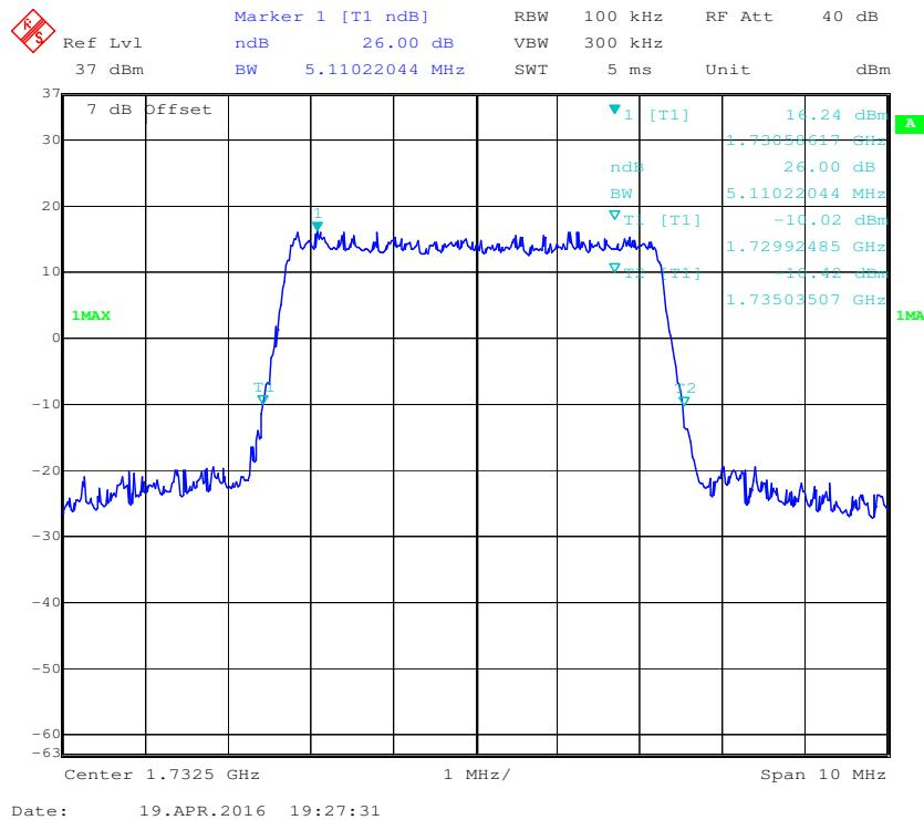
**16-QAM (5.0 MHz) - 99% Occupied Bandwidth, Middle channel**
