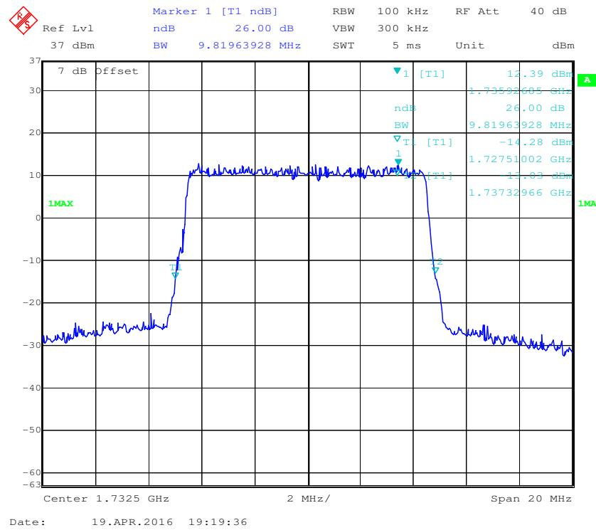
**QPSK (15.0 MHz) - 99% Occupied Bandwidth, Middle channel**
