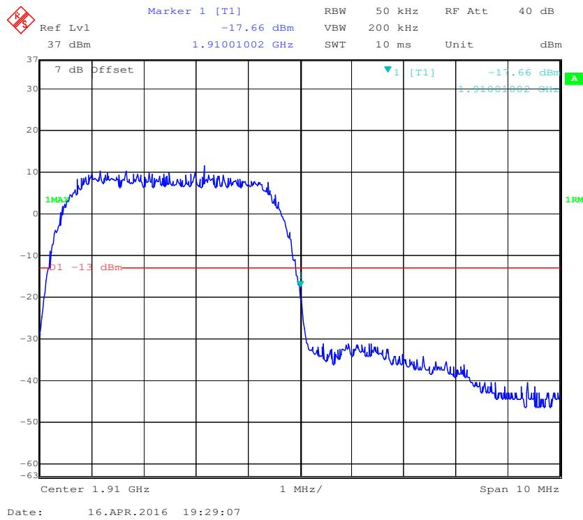
**PCS Band, Left Band Edge for HSDPA (16QAM) Mode**
