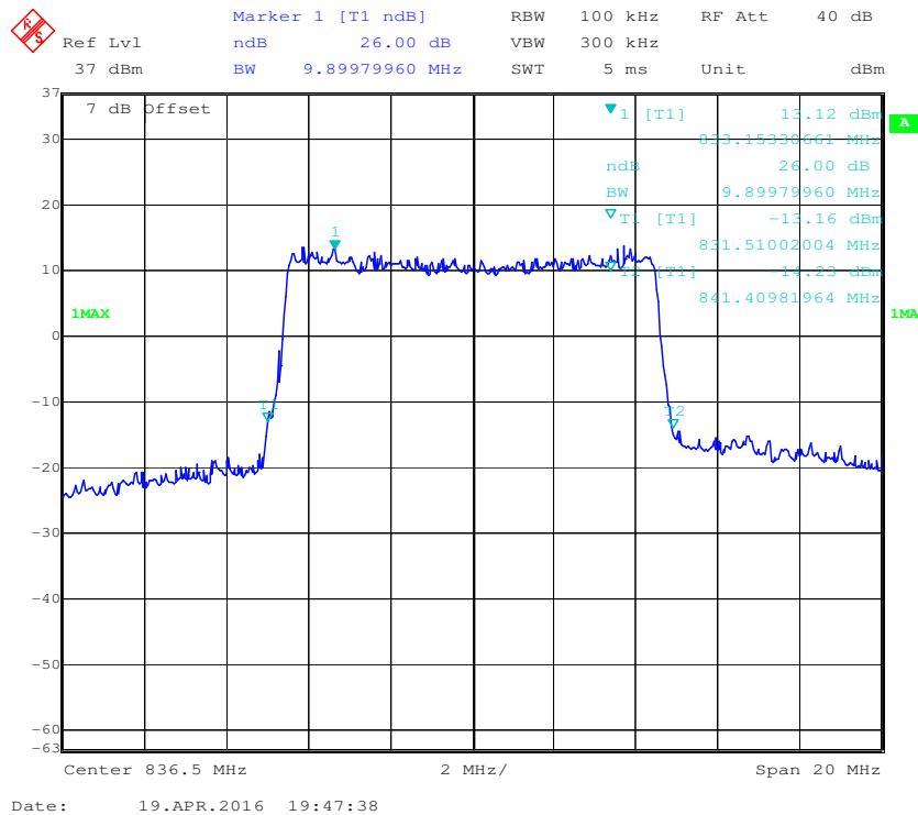
**16-QAM (10.0 MHz) - 99% Occupied Bandwidth, Middle channel**
