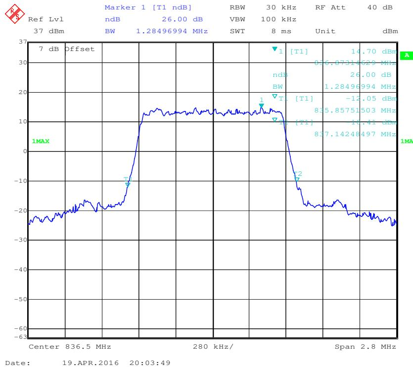
**16-QAM (1.4 MHz) - 99% Occupied Bandwidth Middle channel**
