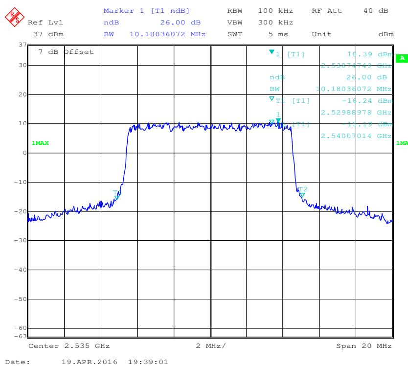
**16-QAM (10.0 MHz) - 99% Occupied Bandwidth, Middle channel**
