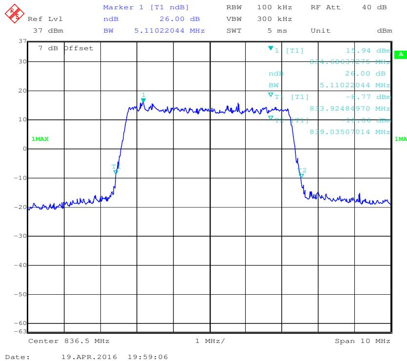
**16-QAM (5.0 MHz) - 99% Occupied Bandwidth, Middle channel**
