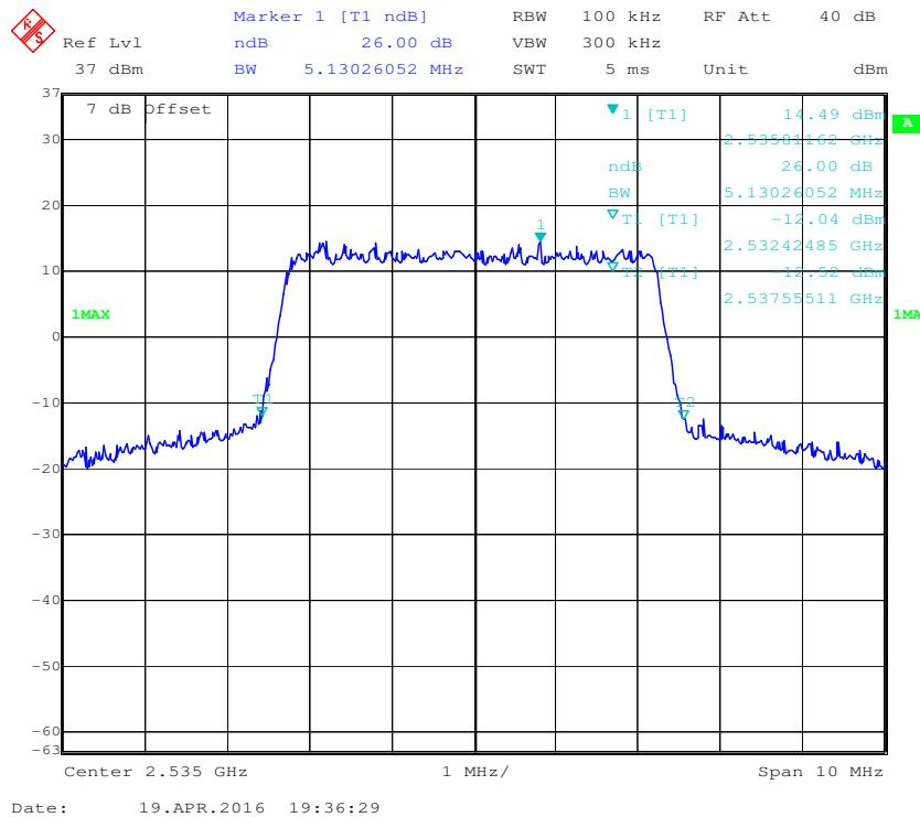
**16-QAM (5.0 MHz) - 99% Occupied Bandwidth, Middle channel**
