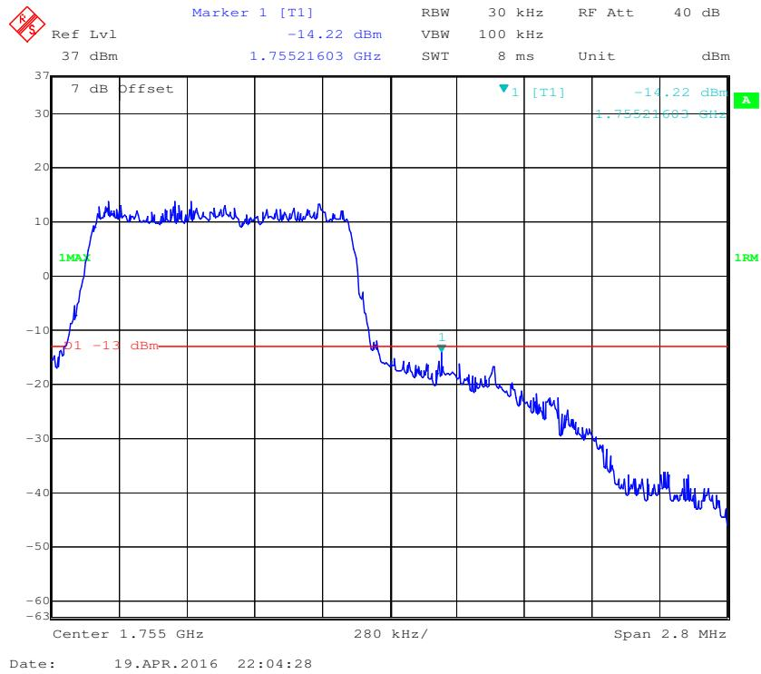
**QPSK (3.0 MHz, FULL RB) - Left Band Edge**
