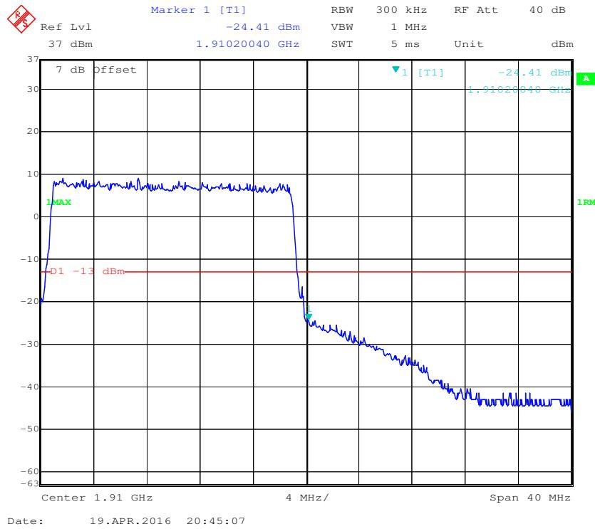
**Band 4:****QPSK (1.4 MHz, FULL RB) - Left Band Edge**
