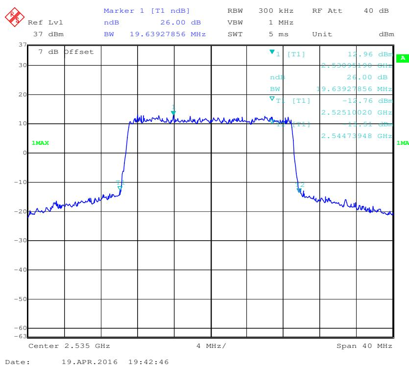
**16-QAM (20.0 MHz) - 99% Occupied Bandwidth, Middle channel**
