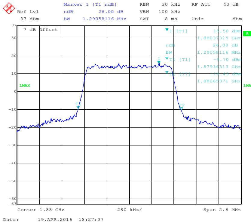
**QPSK (3.0 MHz) - 99% Occupied Bandwidth, Middle channel**
