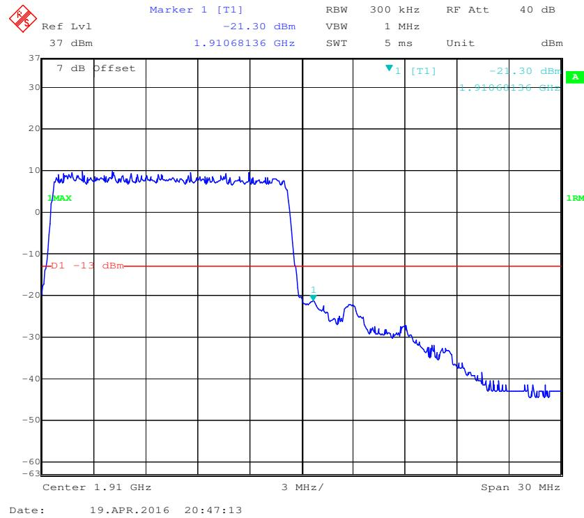
**16-QAM (15.0 MHz, FULL RB) - Left Band Edge**
