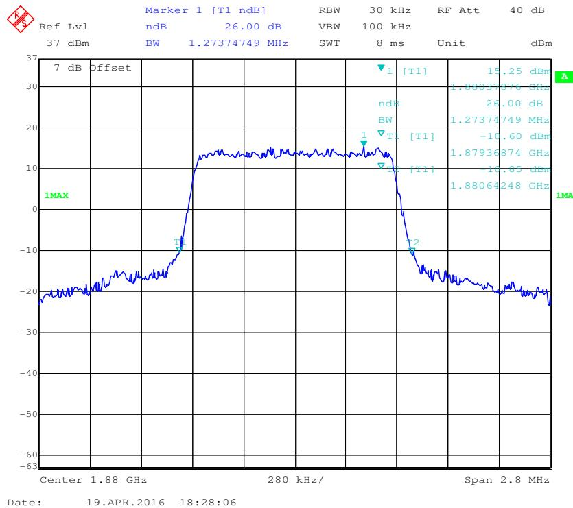
**16-QAM (1.4 MHz) - 99% Occupied Bandwidth Middle channel**
