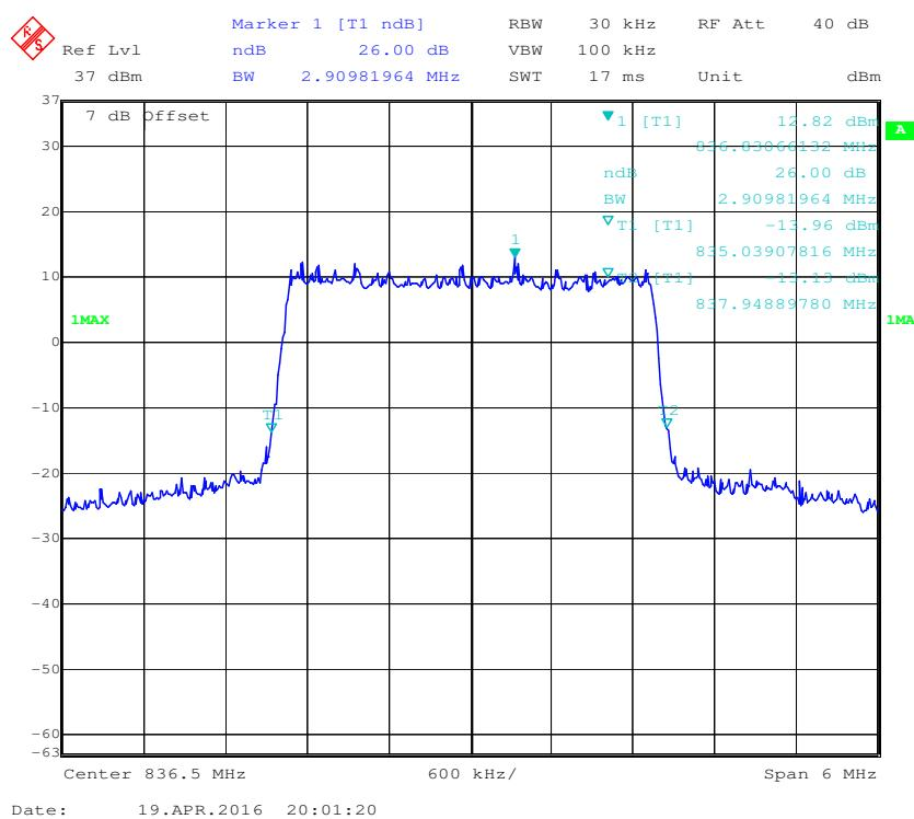
**QPSK (5.0 MHz) - 99% Occupied Bandwidth, Middle channel**
