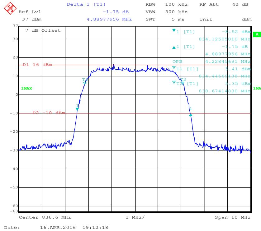
**PCS Band (Part 24E)****99% Occupied & 26 dB Emissions Bandwidth for GSM (GMSK) Mode**
