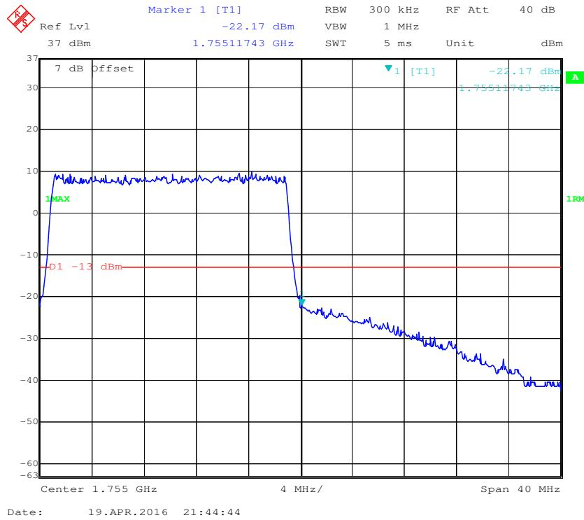
**16-QAM (20.0 MHz, FULL RB) - Left Band Edge**
