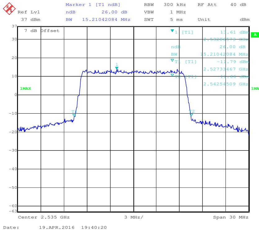
**QPSK (20.0 MHz) - 99% Occupied Bandwidth, Middle channel**
