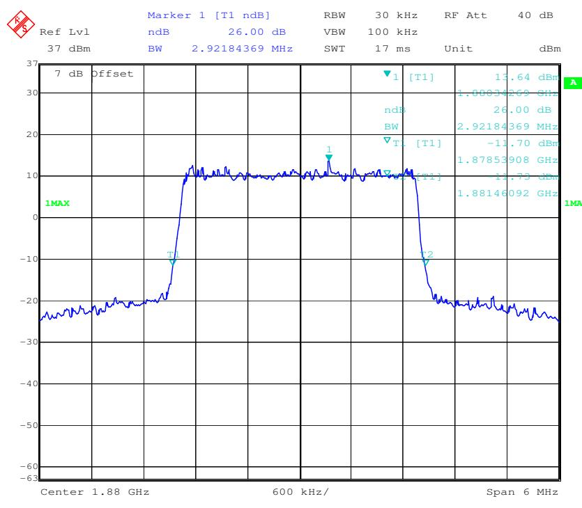
**16-QAM (3.0 MHz) - 99% Occupied Bandwidth, Middle channel**
