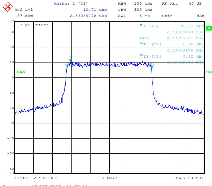
**QPSK (10.0 MHz) - 26 dB Bandwidth, Middle channel**
