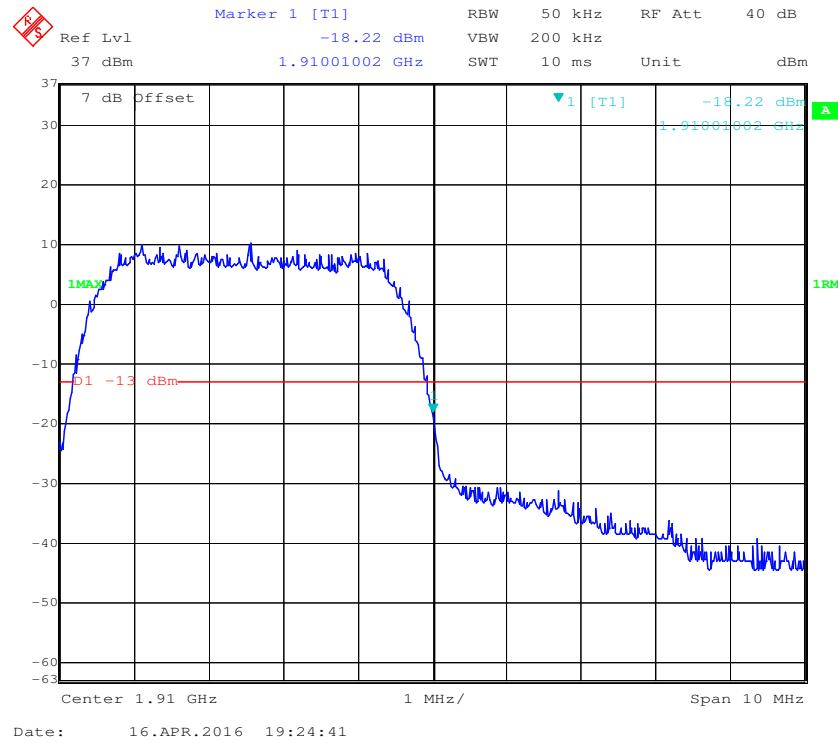
**PCS Band, Left Band Edge for HSUPA (BPSK) Mode**
