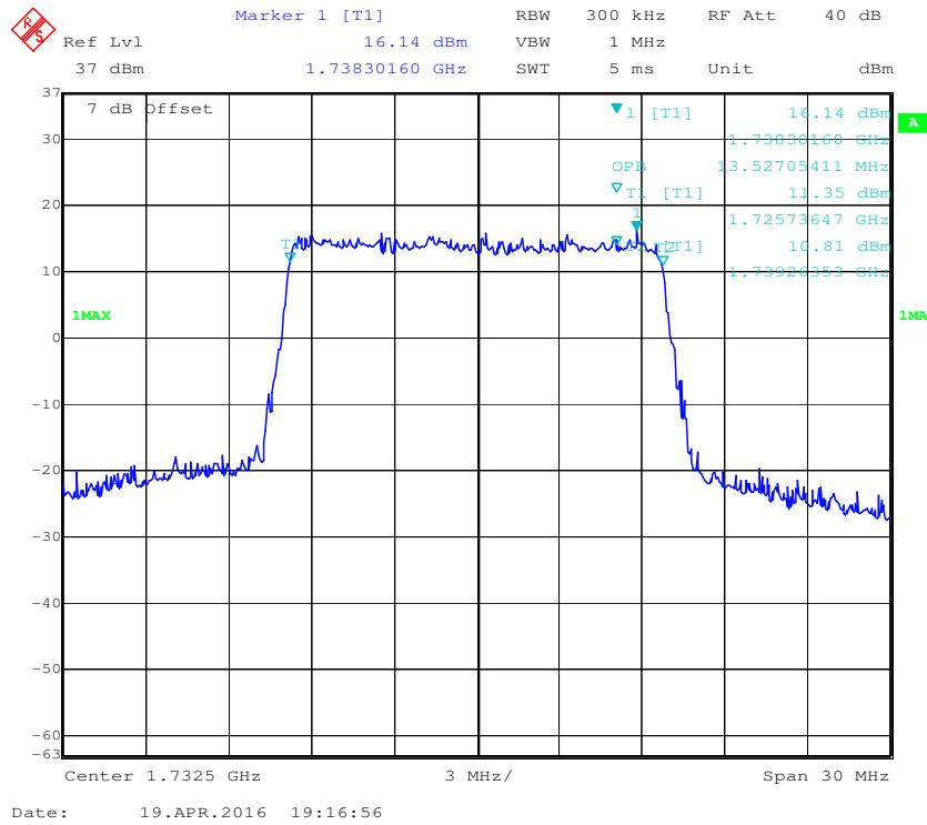
**16-QAM (15.0 MHz) - 26 dB Bandwidth, Middle channel**
