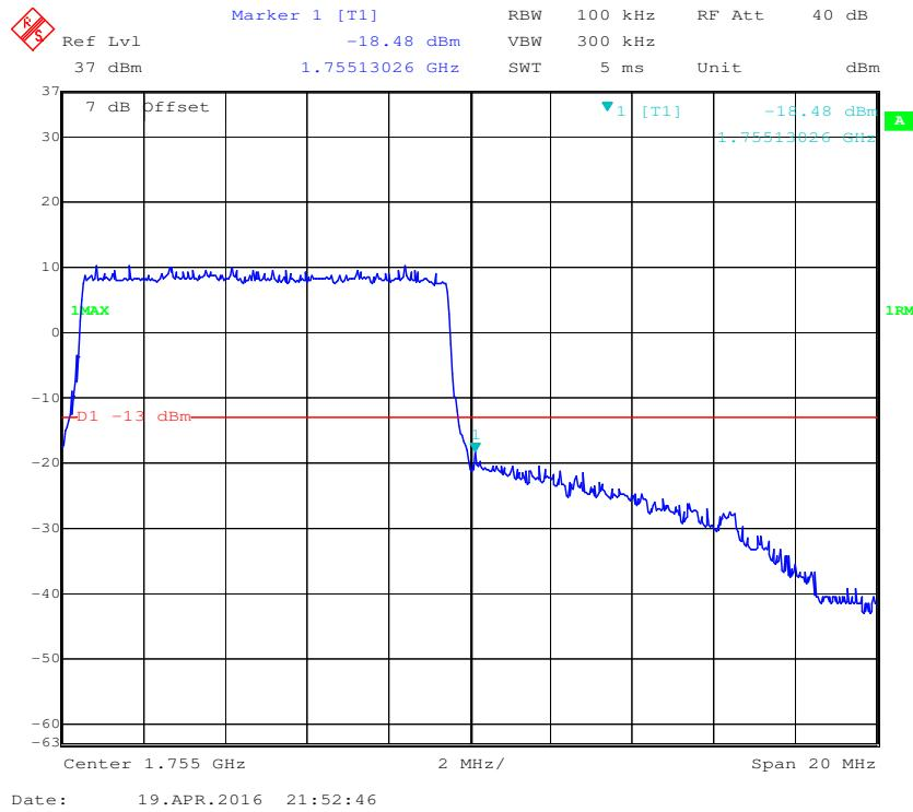
**QPSK (15.0 MHz, FULL RB) - Left Band Edge**
