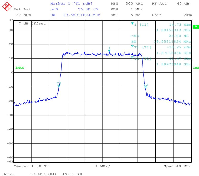
**16-QAM (20.0 MHz) - 99% Occupied Bandwidth, Middle channel**
