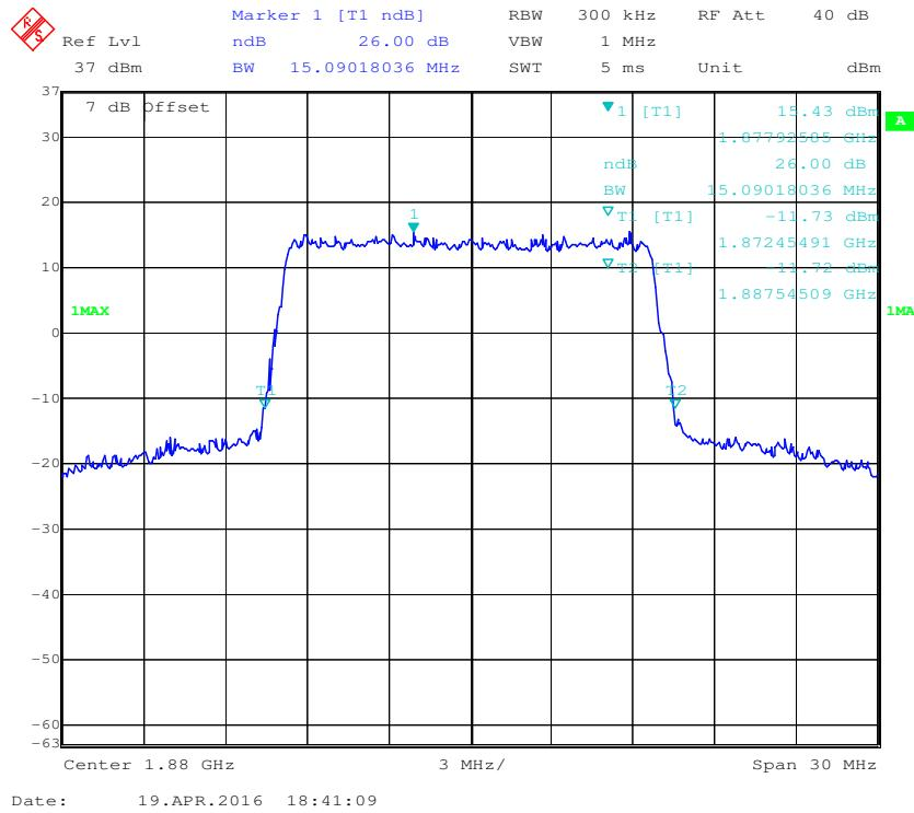
**QPSK (20.0 MHz) - 99% Occupied Bandwidth, Middle channel**
