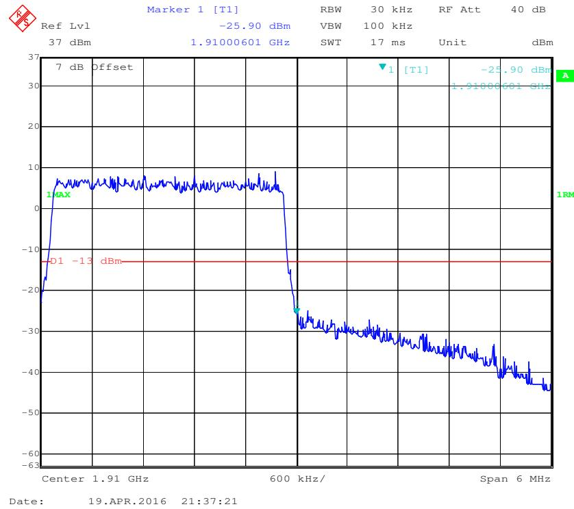
**16-QAM (3.0 MHz, FULL RB) - Left Band Edge**
