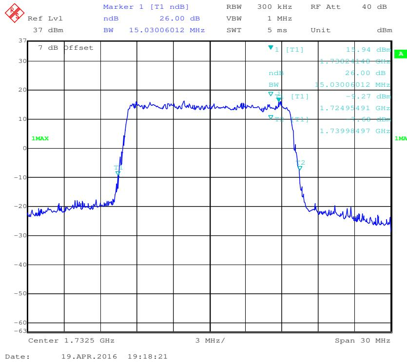
**16-QAM (15.0 MHz) - 99% Occupied Bandwidth, Middle channel**
