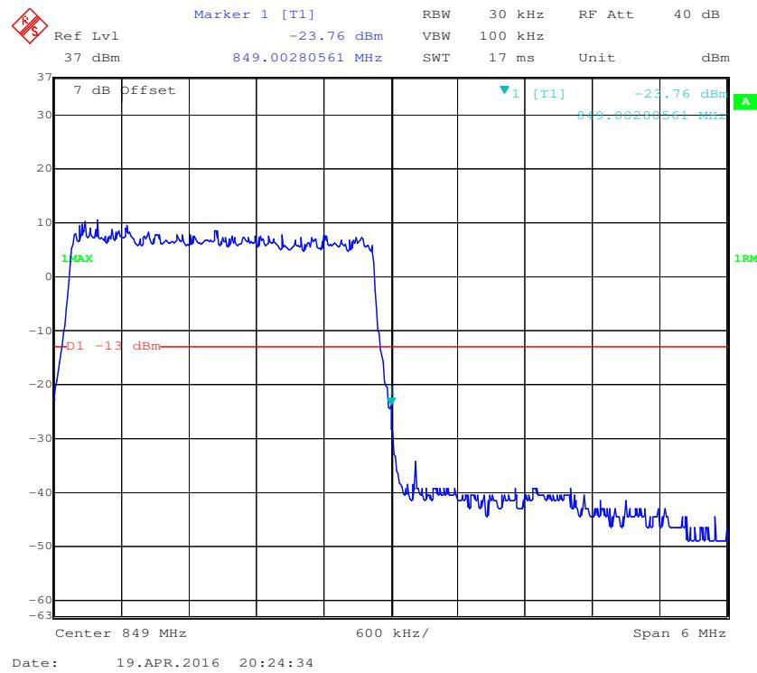
**16-QAM (3.0 MHz, FULL RB) - Left Band Edge**
