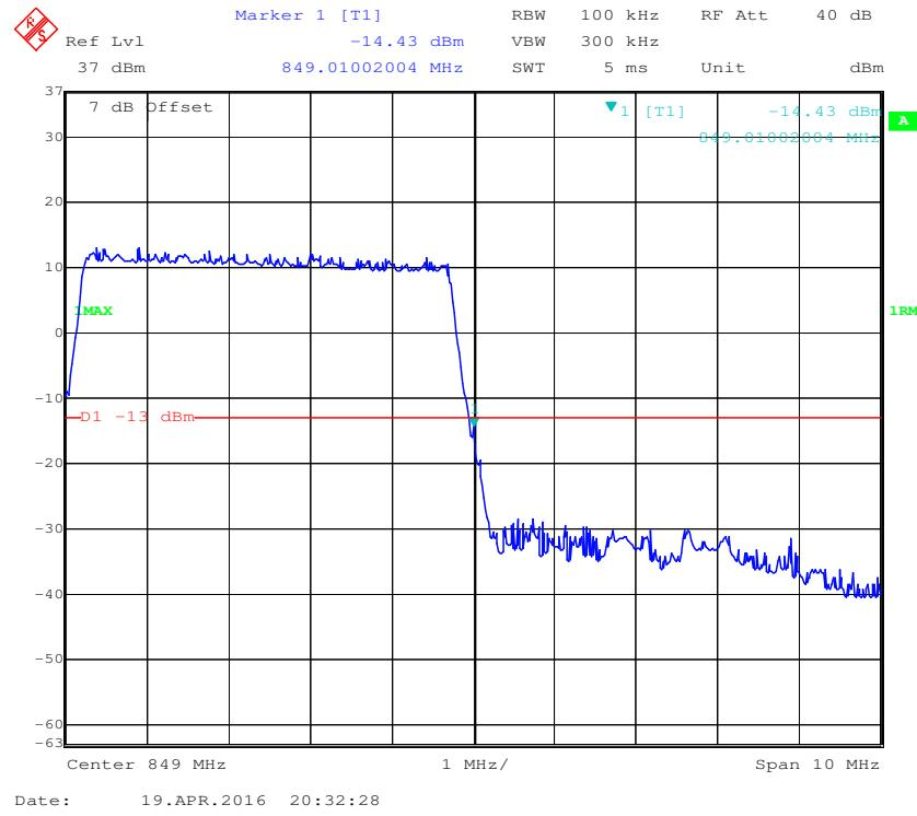
**QPSK (10.0 MHz, FULL RB) - Left Band Edge**
