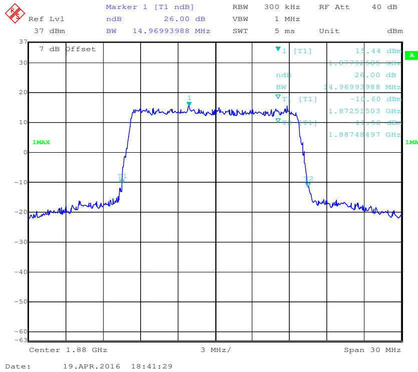
**16-QAM (15.0 MHz) - 99% Occupied Bandwidth, Middle channel**
