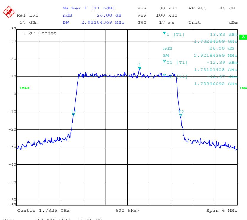
**16-QAM (3.0 MHz) - 99% Occupied Bandwidth, Middle channel**
