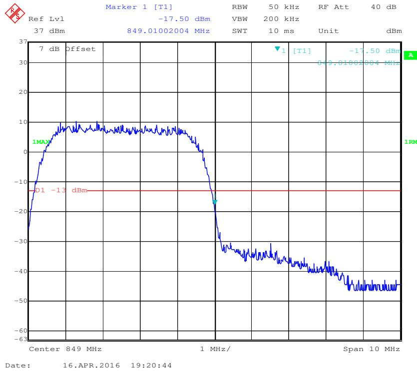
**PCS Band, Left Band Edge for GSM (GMSK) Mode**
