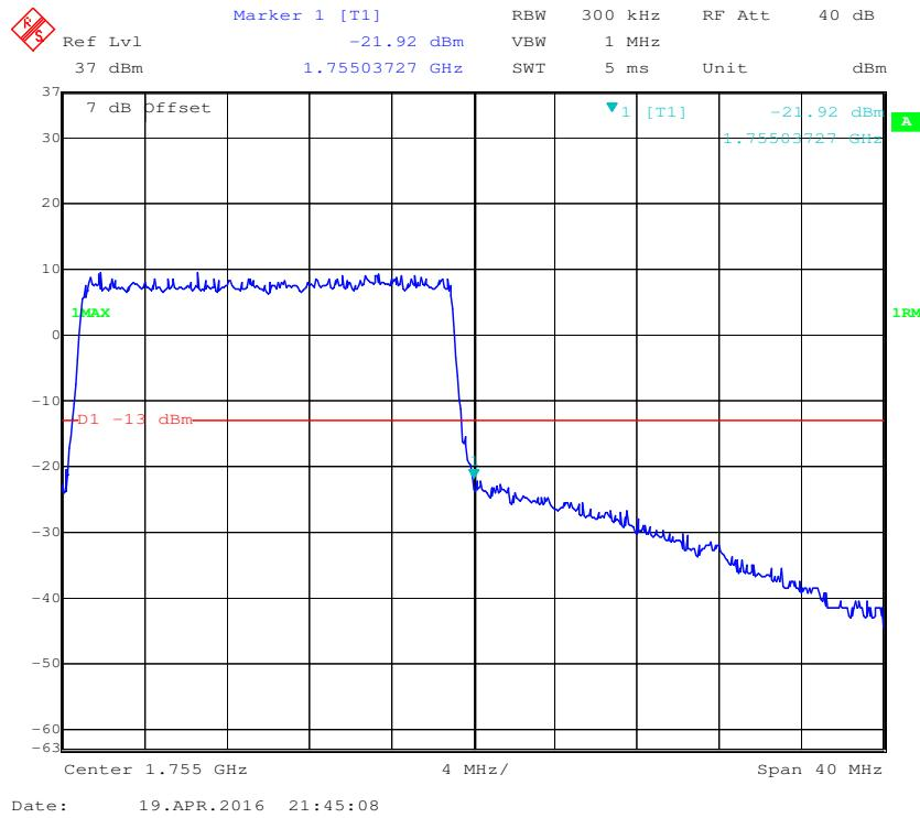
**Band 5:****QPSK (1.4 MHz, FULL RB) - Left Band Edge**
