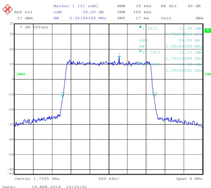
**QPSK (5.0 MHz) - 99% Occupied Bandwidth, Middle channel**
