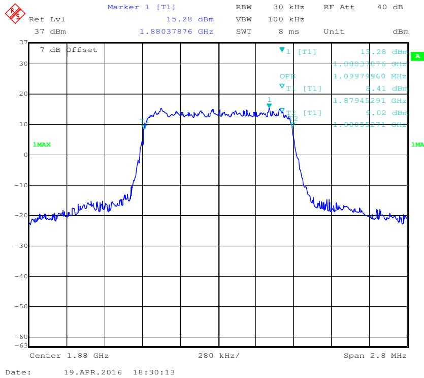
**16-QAM (1.4 MHz) - 26 dB Bandwidth, Middle channel**
