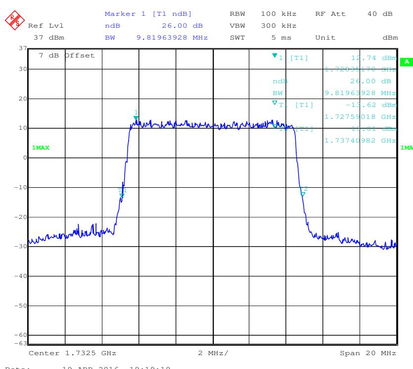
**16-QAM (10.0 MHz) - 99% Occupied Bandwidth, Middle channel**
