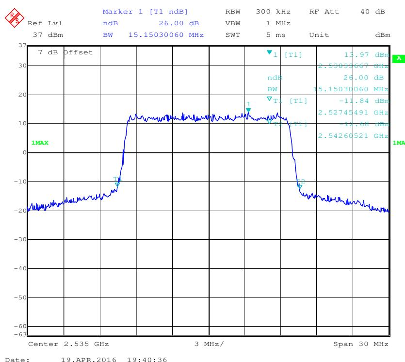
**16-QAM (15.0 MHz) - 99% Occupied Bandwidth, Middle channel**
