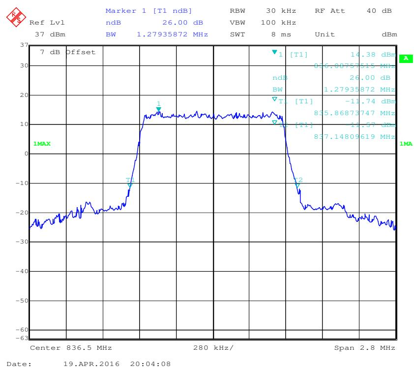
**QPSK (3.0 MHz) - 99% Occupied Bandwidth, Middle channel**
