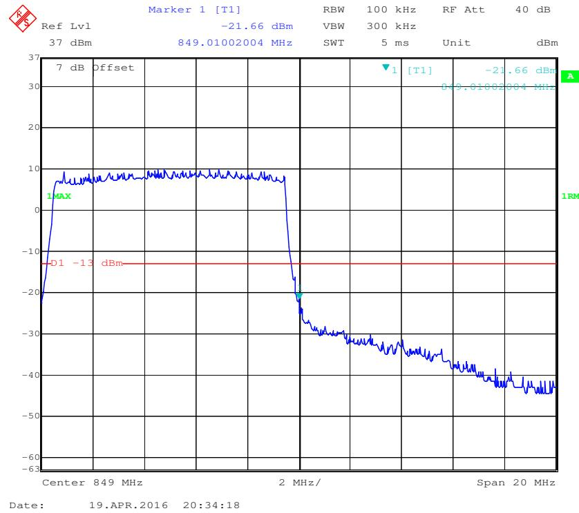
**16-QAM (10.0 MHz, FULL RB) - Left Band Edge**
