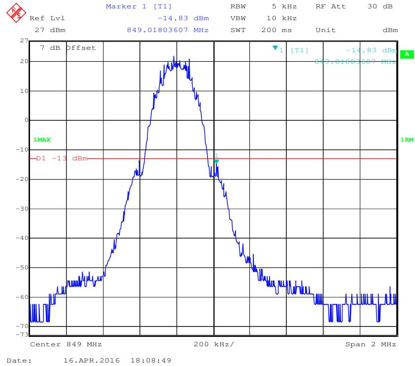
**Cellular Band, Left Band Edge for EGPRS Mode**
