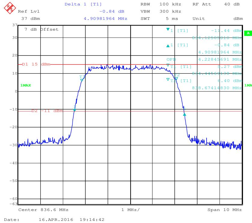
**99% Occupied & 26 dB Emissions Bandwidth for HSDPA (16QAM) Mode**
