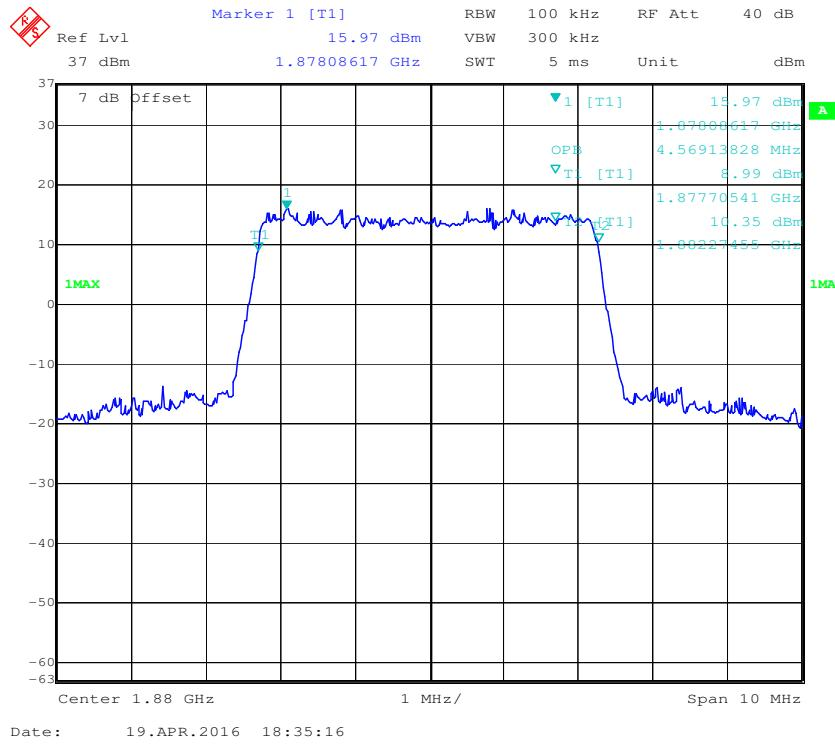
**QPSK (5.0 MHz) - 26 dB Bandwidth, Middle channel**
