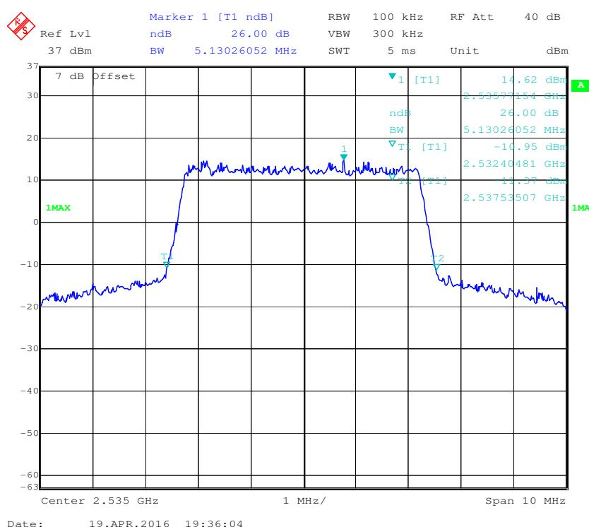
**QPSK (10.0 MHz) - 99% Occupied Bandwidth, Middle channel**
