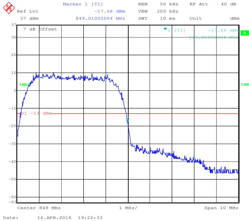
**Cellular Band, Left Band Edge for HSUPA (BPSK) Mode**
