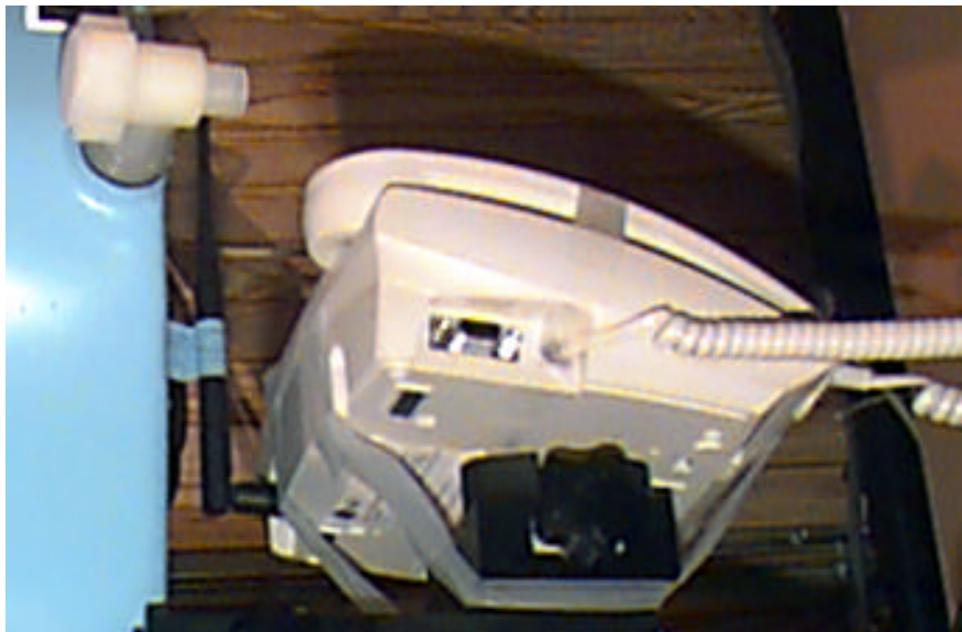
Figure 8. Actual placement of EUT with source of significant emissions placed 2 cm. from phantom surface.
