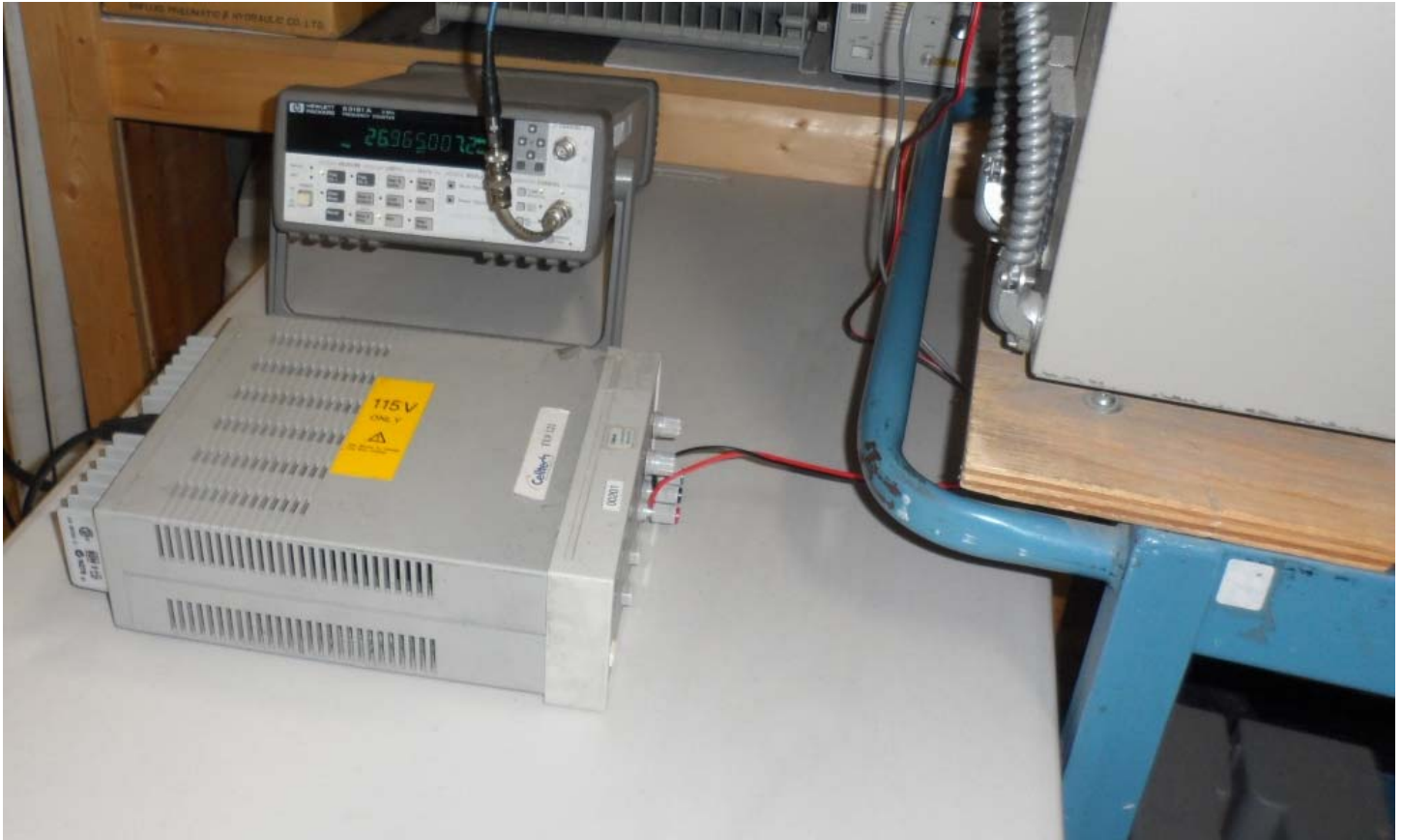
Figure E14.2 – Setup Photo – Frequency Stability - External Equipment
