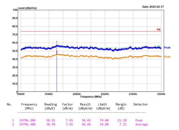
Project No.: 2503Q17178E-RF Tester: Mack Huang Condition: PK trace RBW:1MHz; VBW:3MHz; SWT:0.3sec Polarization: horizontal Note: 2EDR Middle Channel 2441MHz
