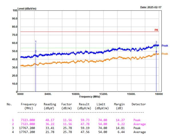
Project No.: 2503Q17178E-RF Tester: Mack Huang Condition: PK trace RBW:1MHz; VBW:3MHz; SWT:0.3sec Polarization: horizontal Note: 3EDR Low Channel 2402MHz
