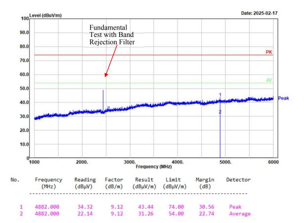
Project No.: 2503Q17178E-RF Tester: Mack Huang Condition: PK trace RBW:1MHz; VBW:3MHz; SWT:0.3sec Polarization: vertical Note: 2EDR Middle Channel 2441MHz
