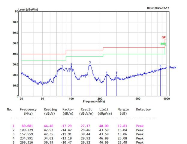
Project No.: 2503Q17178E-RF Tester: Roinin Fu Condition: RBW:100 kHz VBW:300 kHz SWT:0.1 sec Polarization: vertical Note: Transmitting
