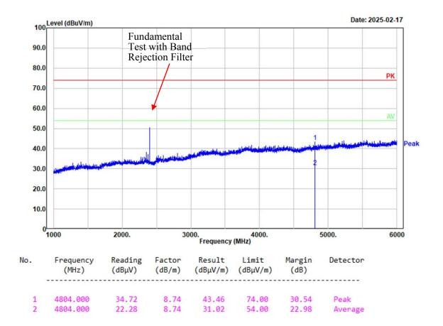
Project No.: 2503Q17178E-RF Tester: Mack Huang Condition: PK trace RBW:1MHz; VBW:3MHz; SWT:0.3sec Polarization: vertical Note: BDR Low Channel 2402MHz
