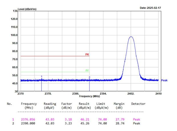
Project No.: 2503Q17178E-RF Tester: Mack Huang Condition: PK trace RBW:1MHz; VBW:3MHz; SWT:0.3sec Polarization: Vertical Note: 3EDR Low Channel 2402MHz
