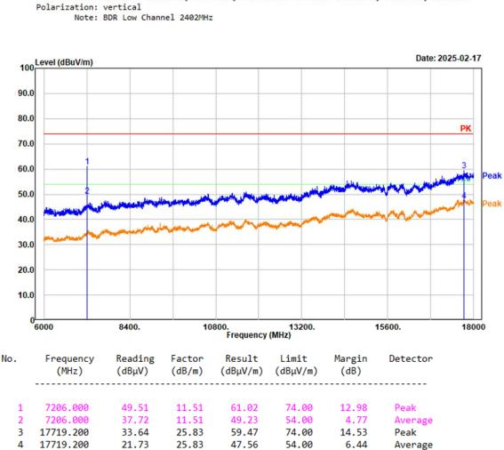
Project No.: 2503Q17178E-RF Tester: Mack Huang Condition: PK trace RBW:1MHz; VBW:3MHz; SWT:0.3sec AV trace RBW:1MHz; VBW:5kHz; SWT:auto Polarization: vertical
