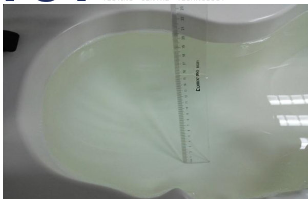
The Head Liquid of 1900MHz (15.5cm)
