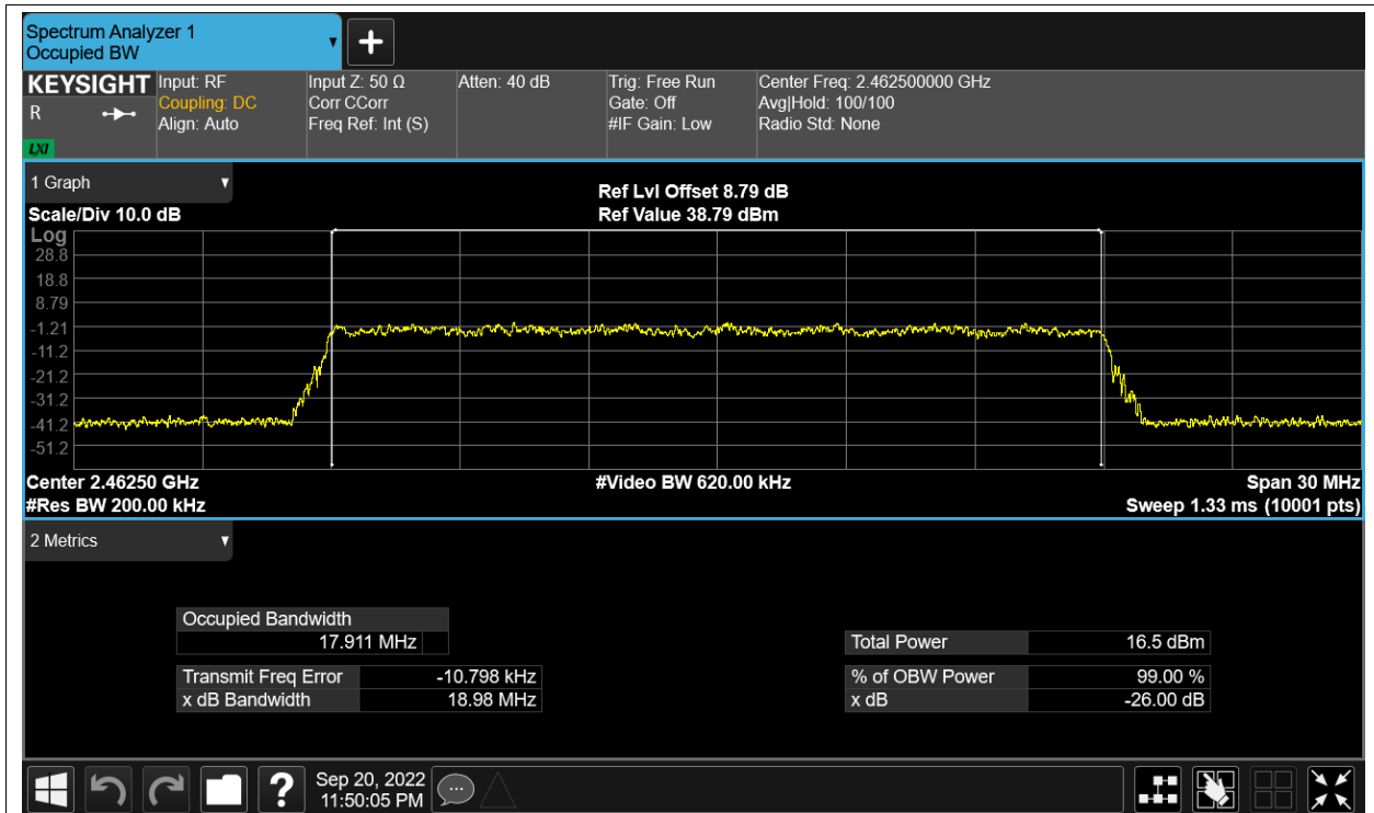
OBW NVNT 2.4G-20M-16QAM 2462.5MHz Ant2
