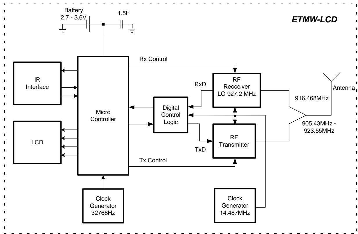
Figure 1: ETMW-LCD Block Diagram
