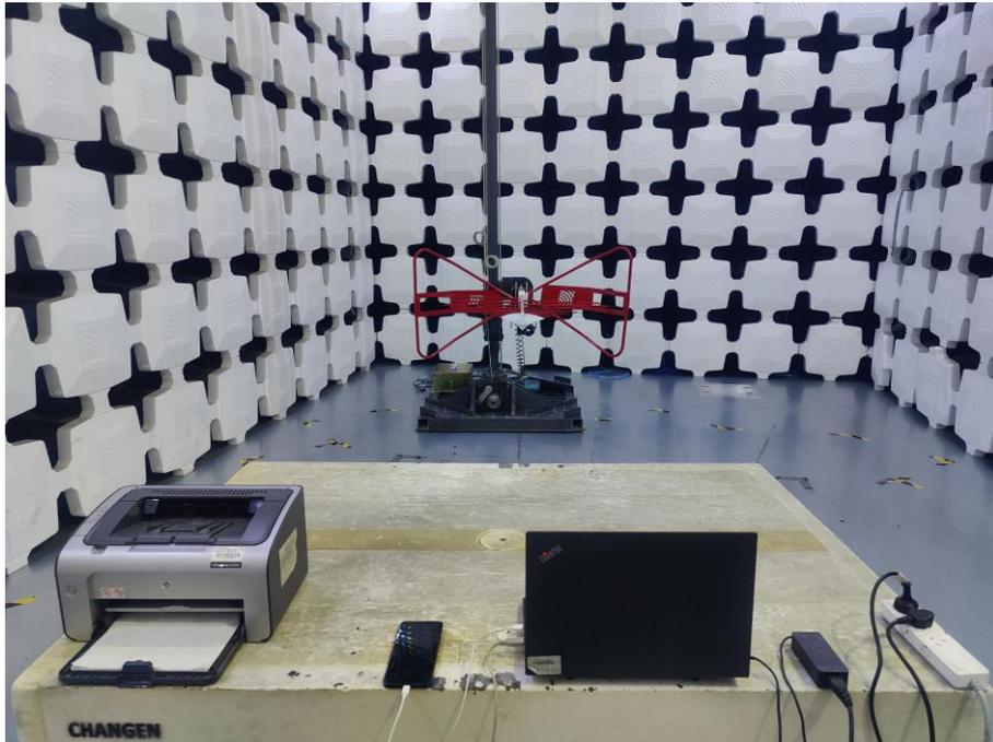
1. Radiated Emissions (Part 15B, Data Transfer, 30MHz-1GHz)
