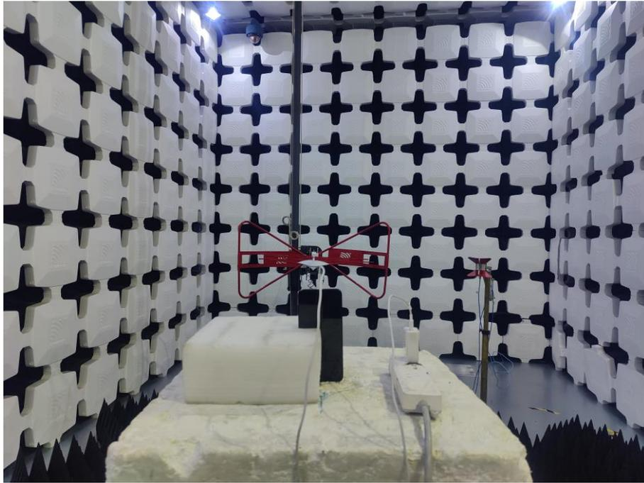
15. Radiated Emissions (Part 15C&Part 15E, 1GHz -18GHz)
