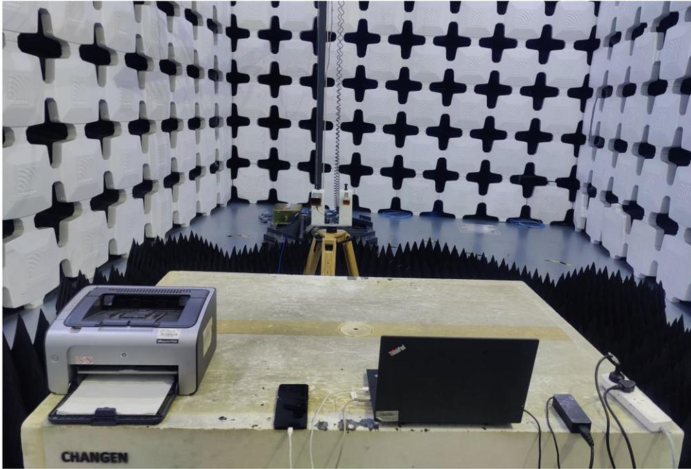
3. Radiated Emissions (Part 15B, Data Transfer, 18GHz-26.5GHz)
