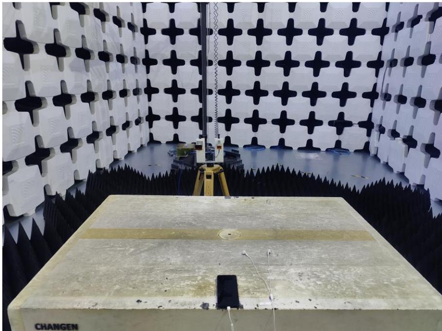
12. Radiated Emissions (Part 15B, FM receiver, 26.5GHz-40GHz)
