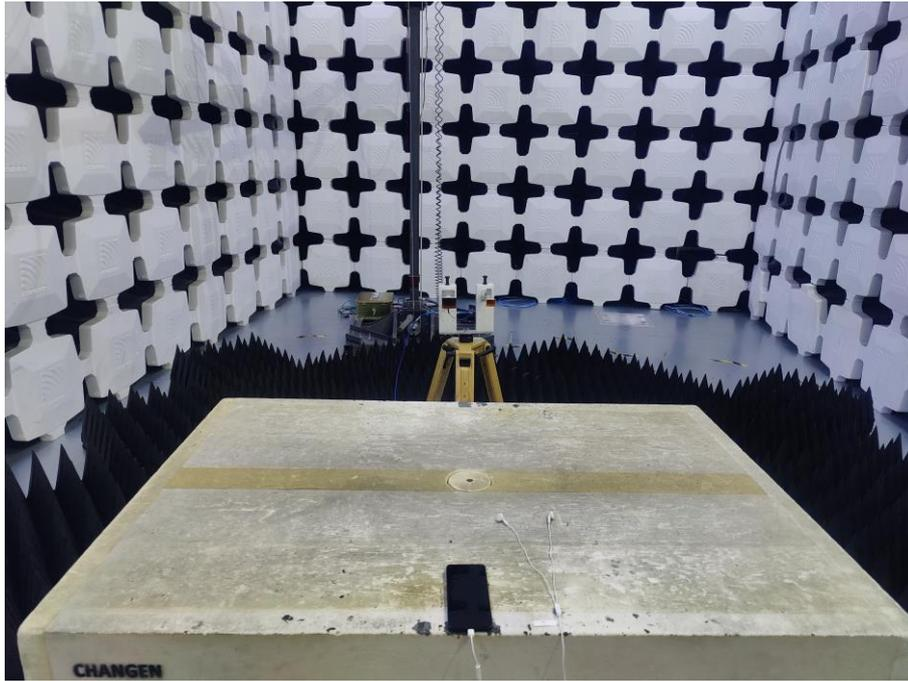
11. Radiated Emissions (Part 15B, FM receiver, 18GHz-26.5GHz)
