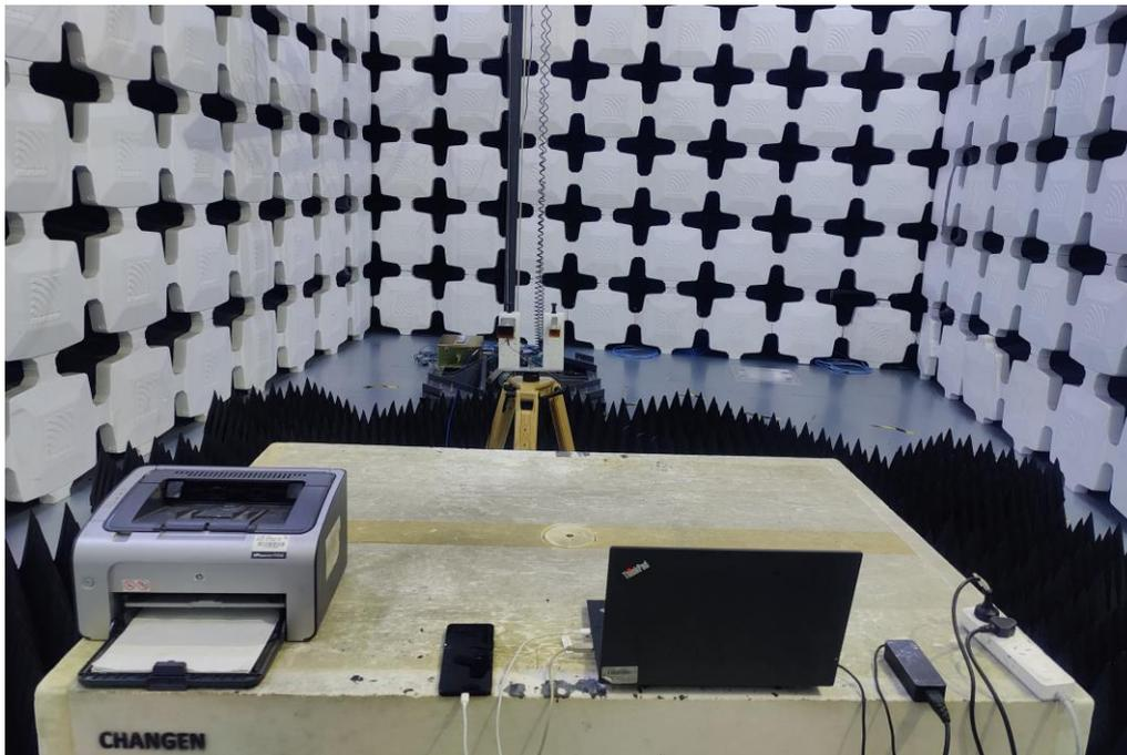
4. Radiated Emissions (Part 15B, Data Transfer, 26.5GHz-40GHz)
