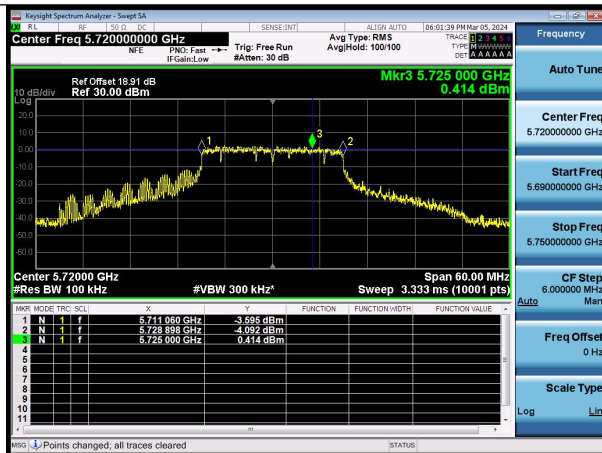
Mode:802.11ac VHT20 Frequency:5720MHz Ant:Chain0 scope:NII2C
