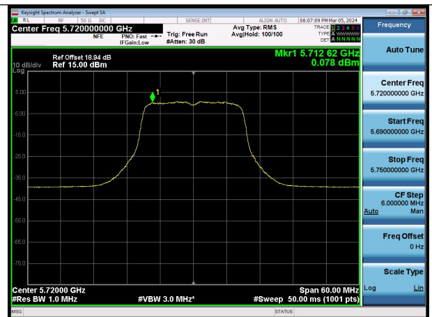
Mode:802.11ac VHT20 Frequency:5720MHz Ant:Chain1 scope:NII2C
