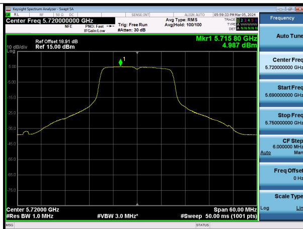
Mode:802.11ac VHT20 Frequency:5720MHz Ant:Chain0 scope:NII2C
