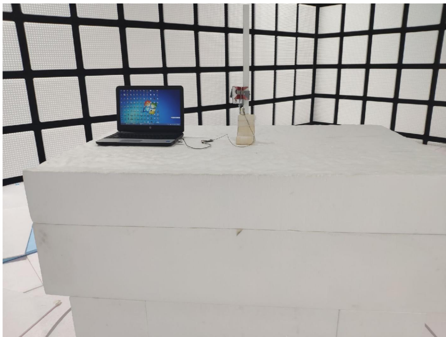
Radiated spurious emission Test Setup-3(Above 1GHz)
