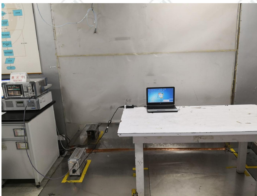
Conducted Emissions Test Setup
