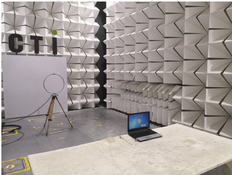
Radiated spurious emission Test Setup-1(Below 30MHz)
