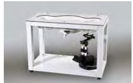
Figure E.5.1 SAM Twin Phantom
