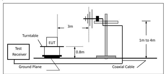
(c) For radiated emissions above 1000MHz
