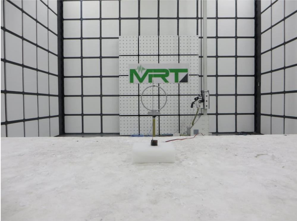
Description: Radiated Emission Test Setup for 30MHz ~ 1GHz (SPM9746) (0.8m Height)
