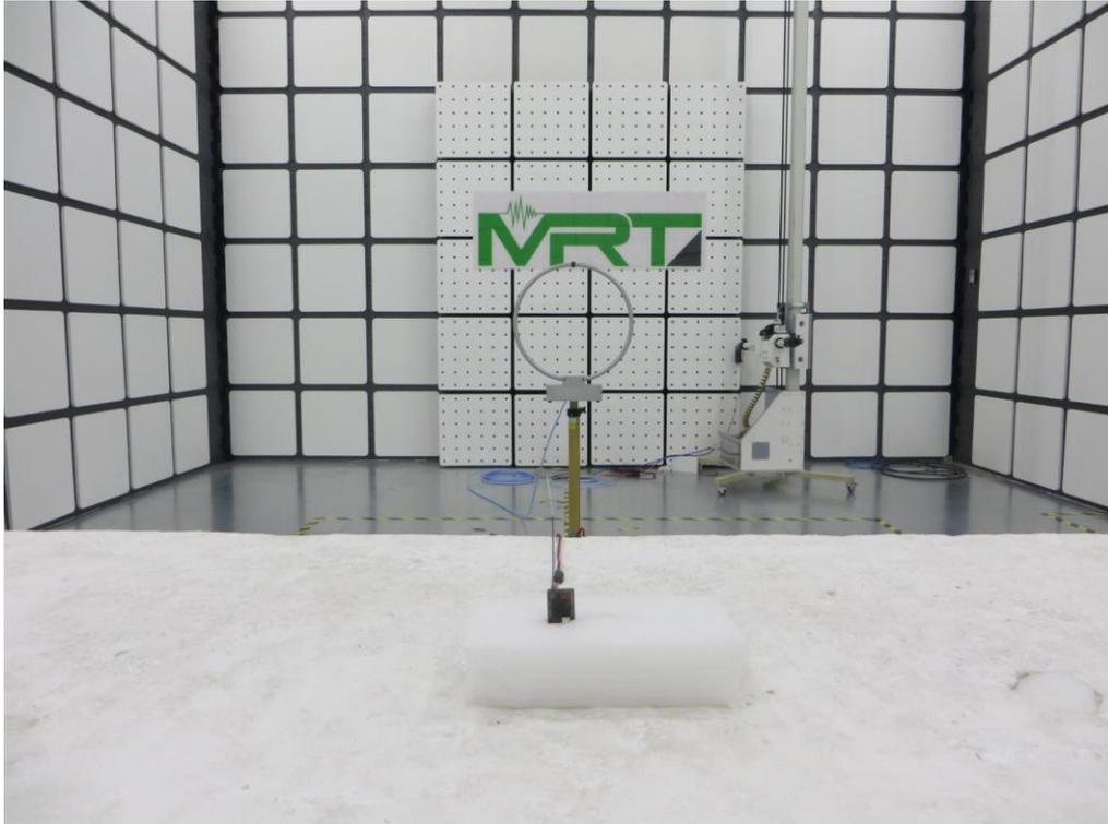
Description: Radiated Emission Test Setup for 30MHz ~ 1GHz (SPM9745) (0.8m Height)
