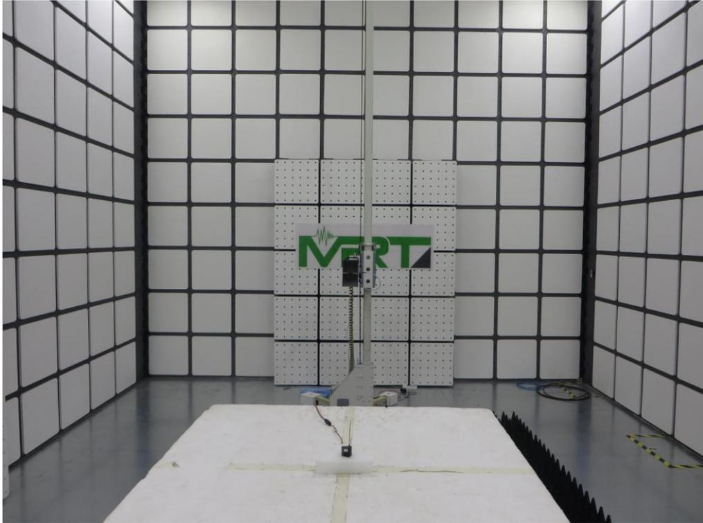
Description: Radiated Emission Test Setup for 18GHz ~ 25GHz (SPM9745) (1.5m Height)
