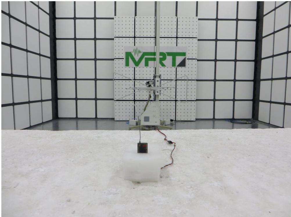
Description: Radiated Emission Test Setup for 1GHz ~ 18GHz (SPM9745) (1.5m Height)
