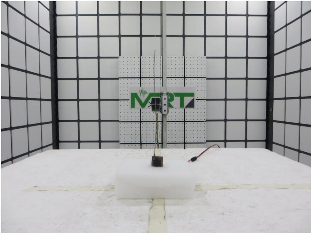
Description: Radiated Emission Test Setup for 18GHz ~ 25GHz (SPM9746) (1.5m Height)
