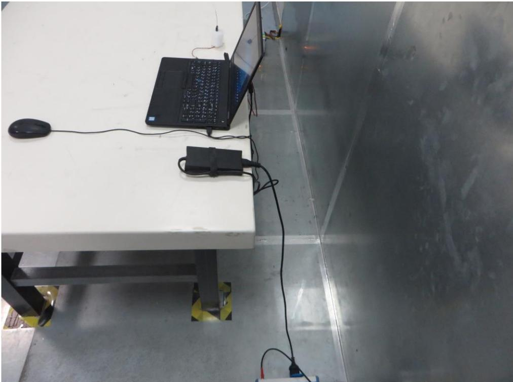
Description: Radiated Emission Test Setup for 9kHz ~ 30MHz (SPM9745) (0.8m Height)
