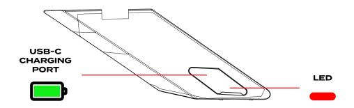
Plug the USB-C cable into the charging port, the LED will light up **RED** and stay static to indicate it is charging.
