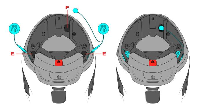
**3.** Carefully re-attach the cheek pads over the top of the speakers and Mic cable.
