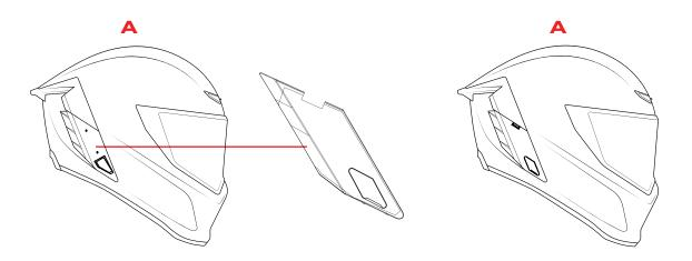
**3.** Insert Shockwave into side [B] by lining up the locators with slots in the Shockwave cavity, and press until it 'CLICKS'.
