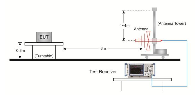
Above 1GHz Test Setup:
