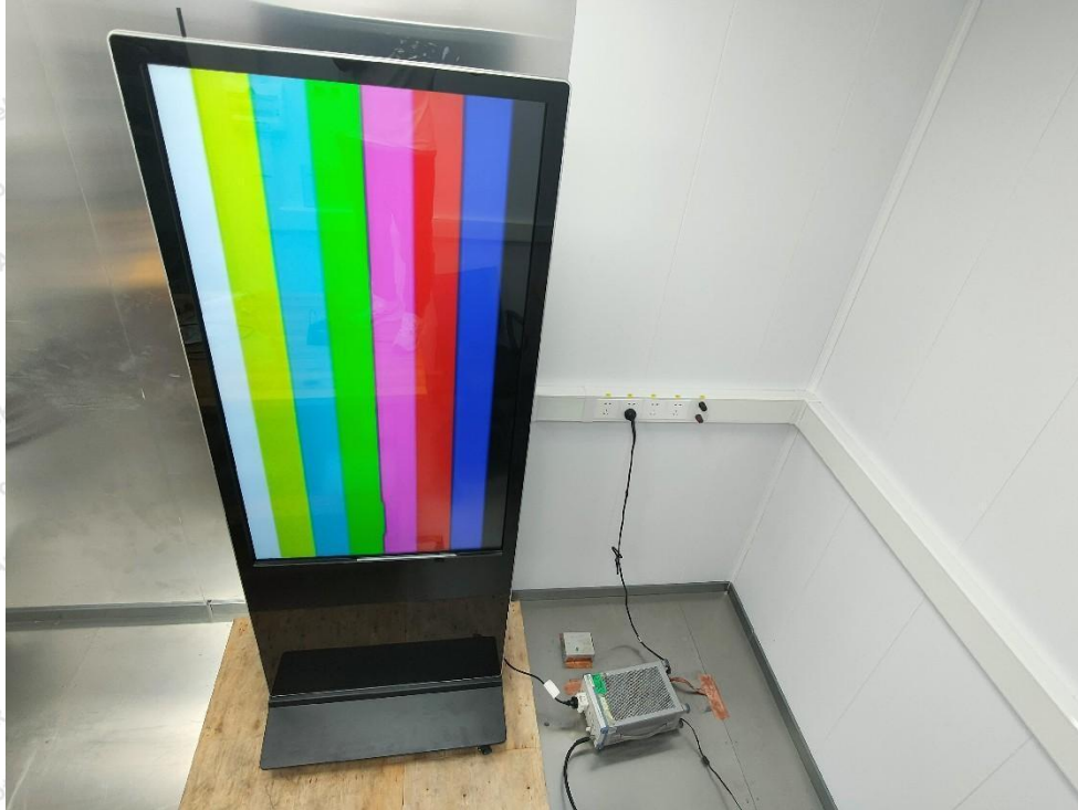
Photo of Radiation Emission Test (below 1GHz)
