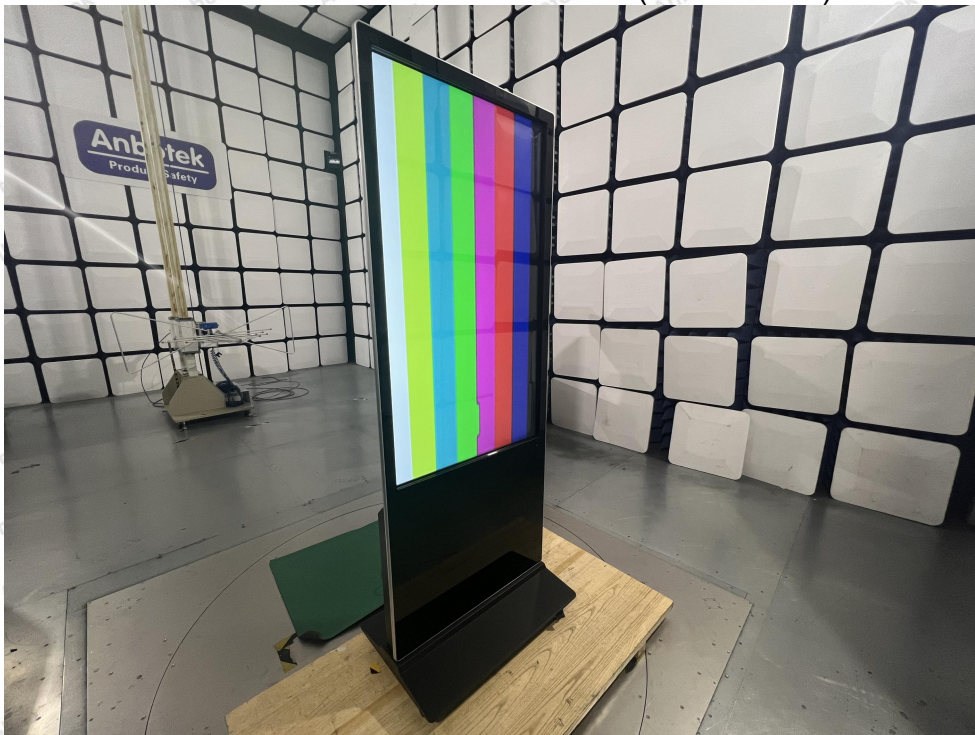
Photo of Radiation Emission Test (below 1GHz)
