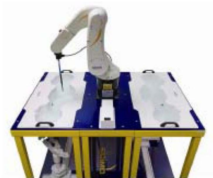
The EUT under test operating at the maximum power level is placed in the phone holder, under the phantom, which is filled with head simulating liquid. The E-Field probe measures the electric field inside the phantom. The OpenSAR software computes the results to give a SAR value in a 1g or 10g mass.
