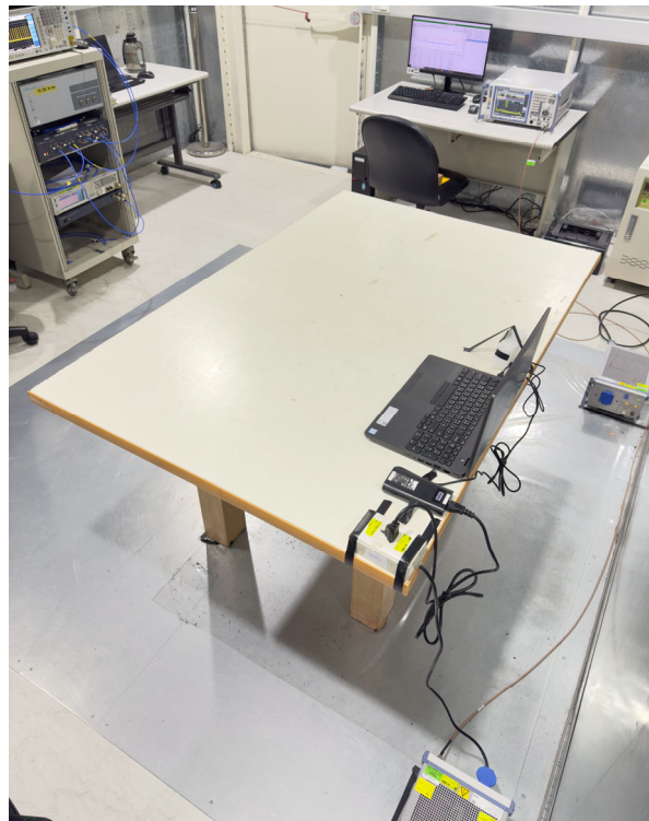
Back View of AC Power Line Conducted Emission Test
