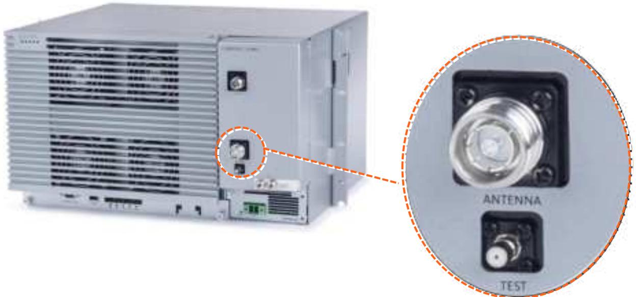
*Note: The test port is used for coupling; used for measuring the power without disconnecting the antenna.*
