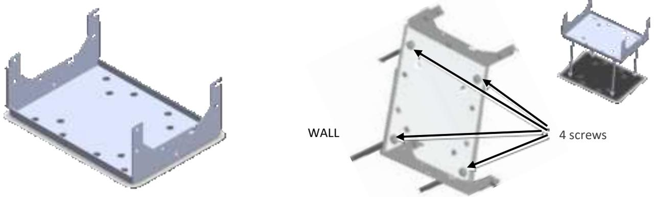
2. For a single unit: mount the LRU on the bracket, using 4 screws
