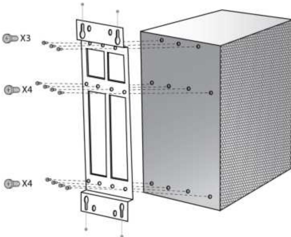
3. Insert anchors in wall, hang unit and tighten to secure
