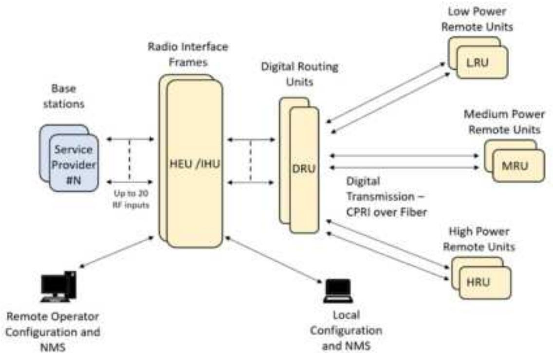
Corning Everon™ 6000 allows combining between Optical Network Evolution (ONE) platform, and the fully digital Corning Building Wireless System (BWS) platform, which incorporates the digital distribution units – Digital Router Unit (DRU) and remotes.
