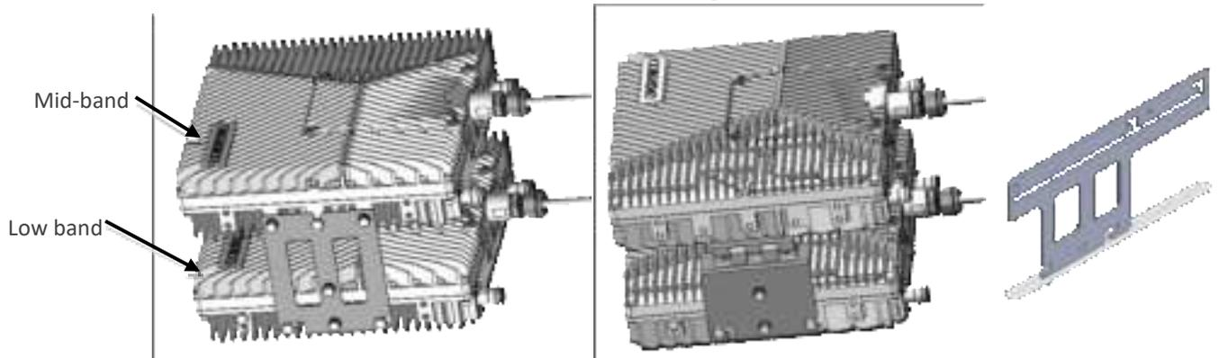
*Note: Ensure the low band device is connected at the bottom, and the mid-band on top!*
