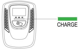
Waiting for Charging - Green Light After the vehicle connector is connected to the vehicle inlet, the CHARGE light is constantly lit.
