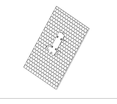
Step 2: Align the rear notch of charger into the wall-mounted bracket and fit the screw holes of the right and left side.
