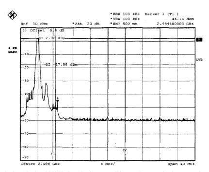
Observation: All emissions in the 100kHz band edge are all lower than carrier by more than 20dB.
