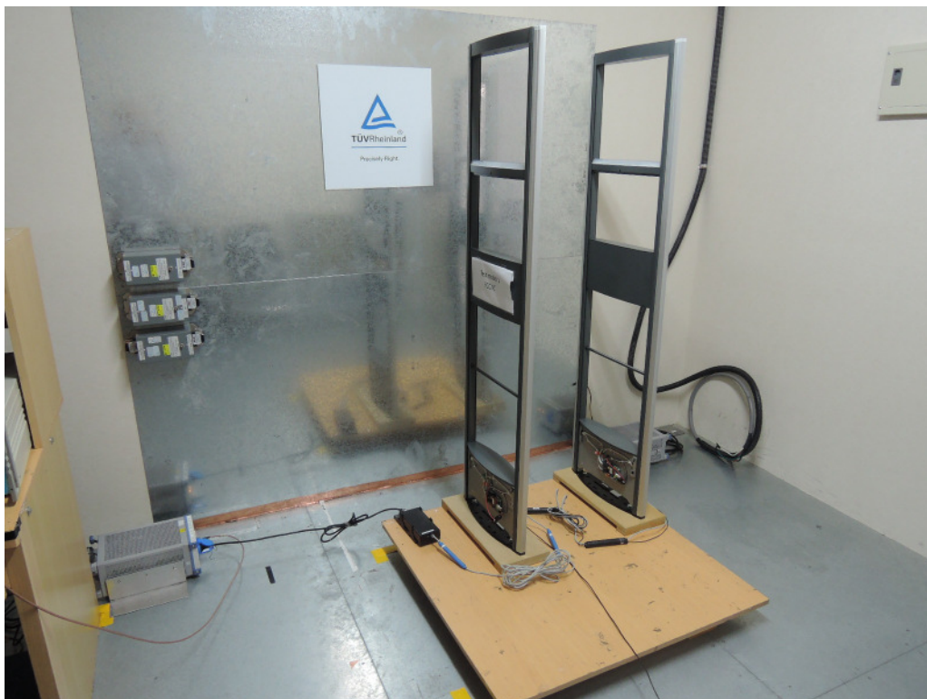
Photograph 5: Set-up for for Mains Conducted testing Front
