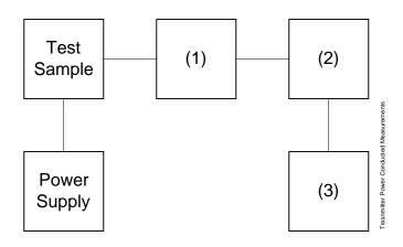
Asset Description s/n (as applicable) (1) COAXIAL ATTENUATOR i00122 Narda 766-10 7802 i00123 Narda 766-10 7802A i00069 Bird 8329 (30 dB) 1006 i00113 Sierra 661A-3D 1059 (2) POWER METERS i00014 HP 435A 1733A05836 i00039 HP 436A 2709A26776 i00020 HP 8901A POWER MODE 2105A01087
