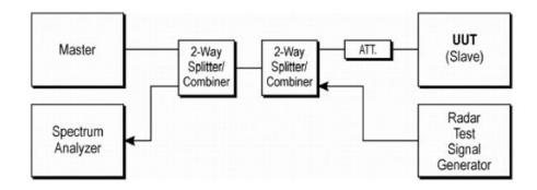
Figure 3-1. Conducted Test Setup for DFS
