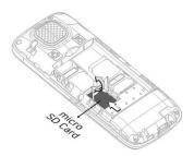
Place back the battery and back cover of the GSM Mobile Phone.
