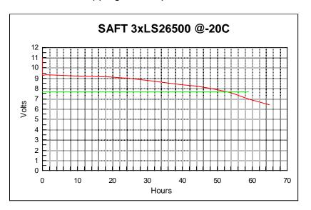
The result achieved was 52.4 hours to 7.7V. However, placing the radiating beacon in the environmental chamber increases the current from 48mA to 53mA which means the actual result if measured in free space would be (52.4x53/48=) 57.8 hours. (See original report).
