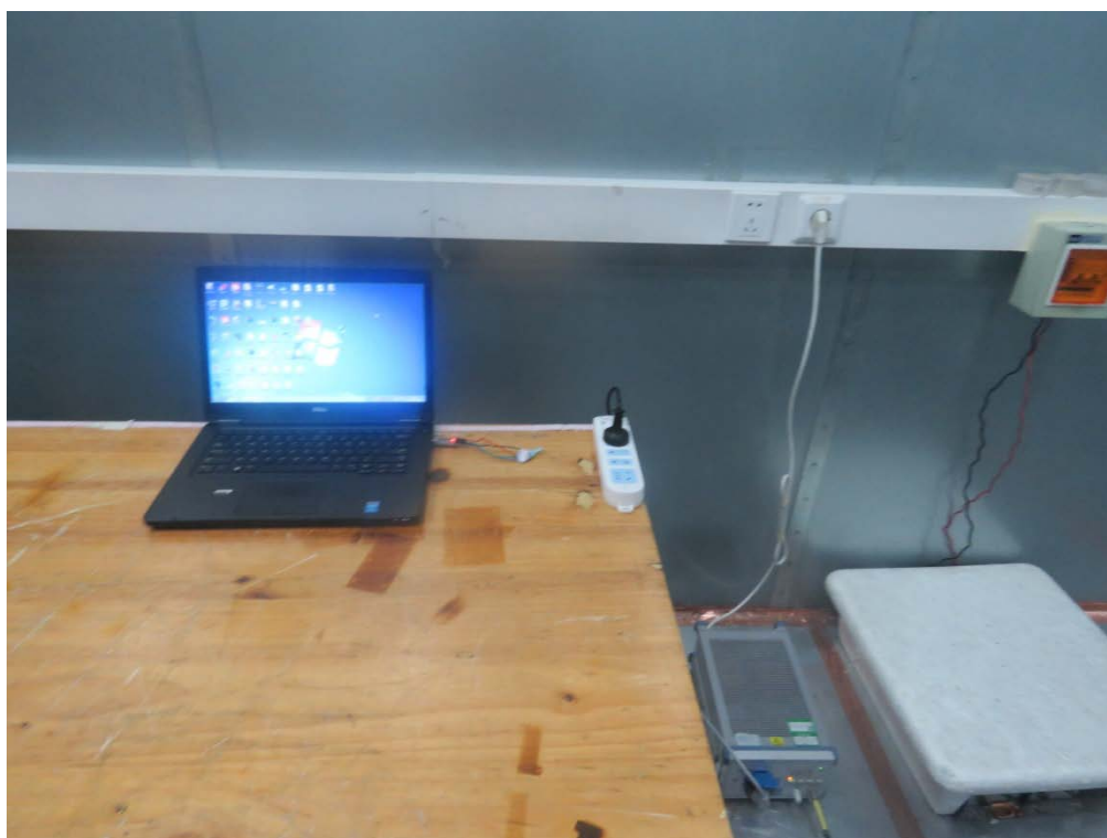
Picture 2 Conducted Emission Test Setup
