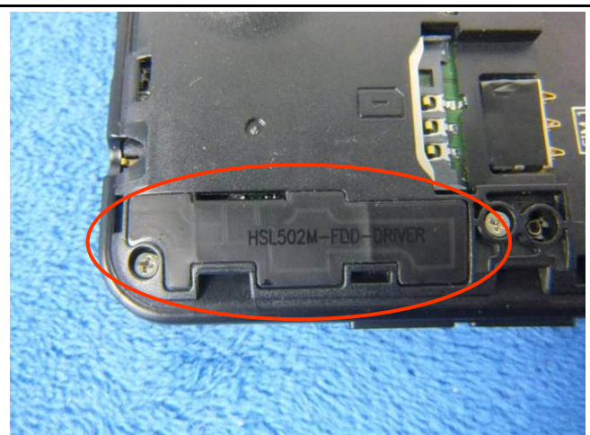
LTE - Antenna View
