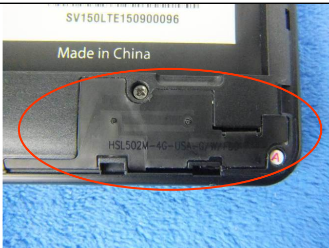
GSM/PCS/UMTS-FDD Antenna View
