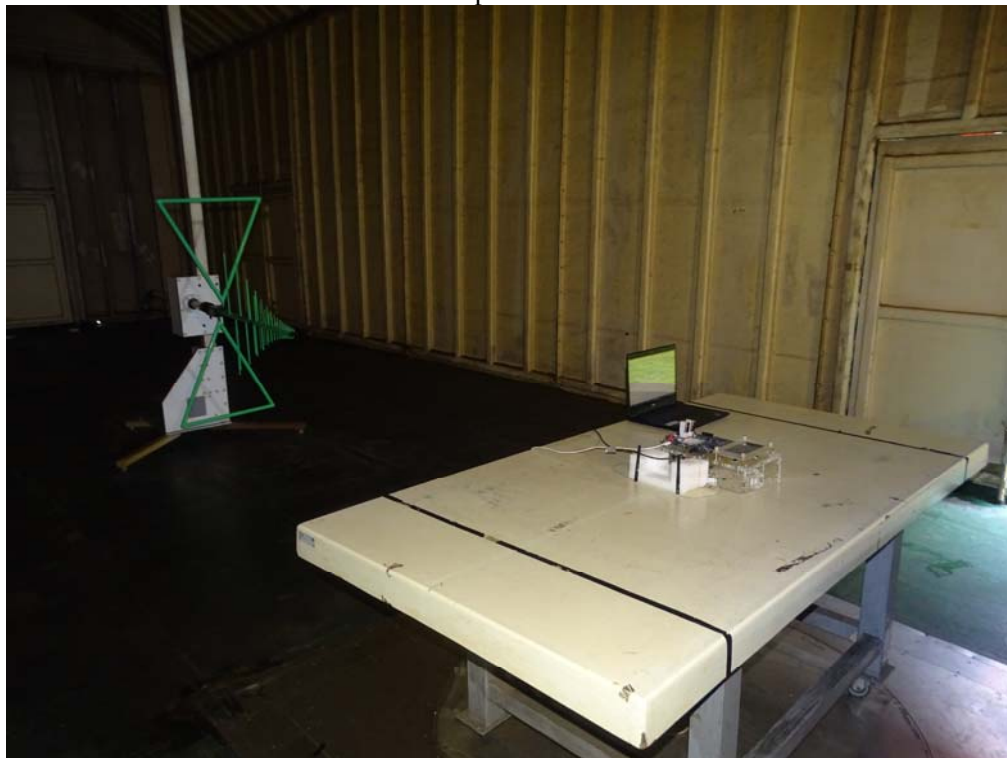
Front View of Spurious Emission Test
