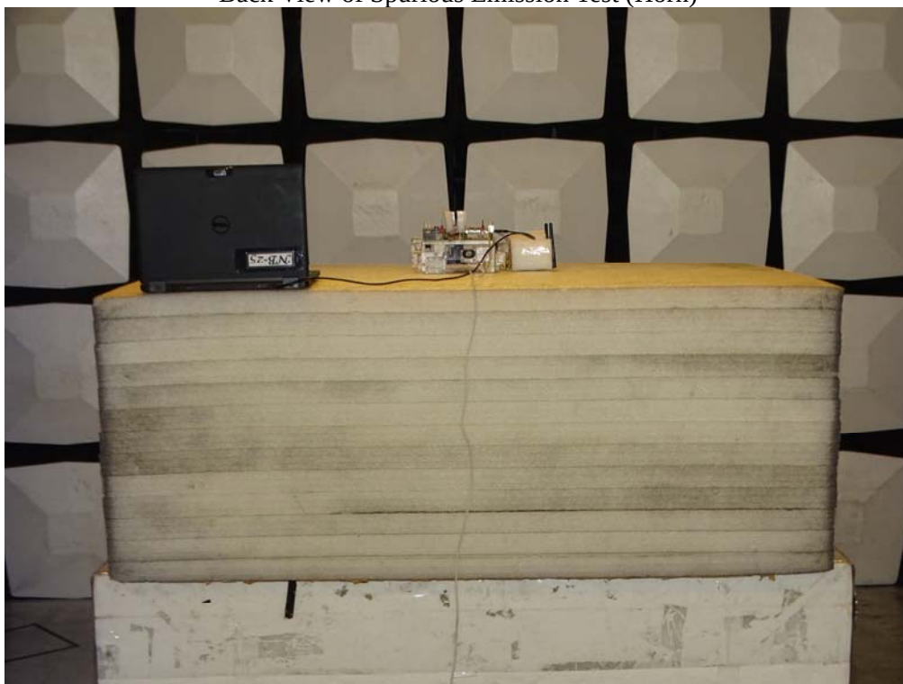
Back View of Spurious Emission Test (Horn)
