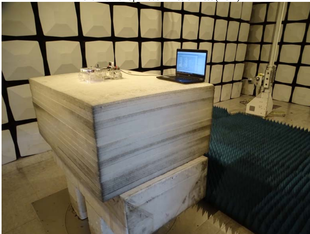
Back View of Spurious Emission Test (Horn)
