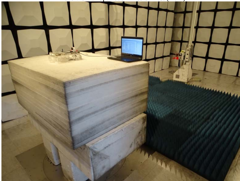
Back View of Spurious Emission Test (Horn)
