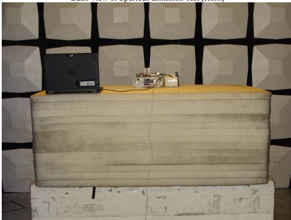
Back View of Spurious Emission Test (Horn)
