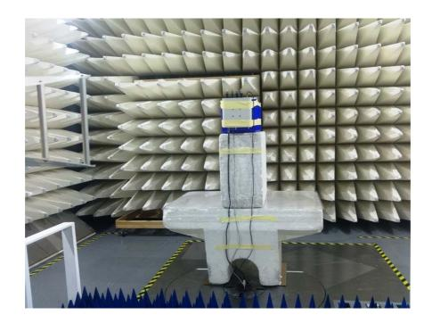
$\label{eq:Photograph No.6} Photograph No.6 \\ Spurious emissions measurement setup in the anechoic chamber in 18 – 37 GHz$
