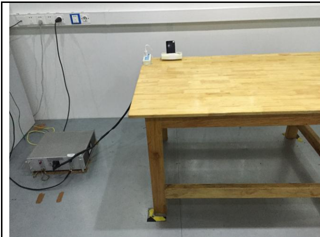
Conducted Emissions Test Setup Front View
