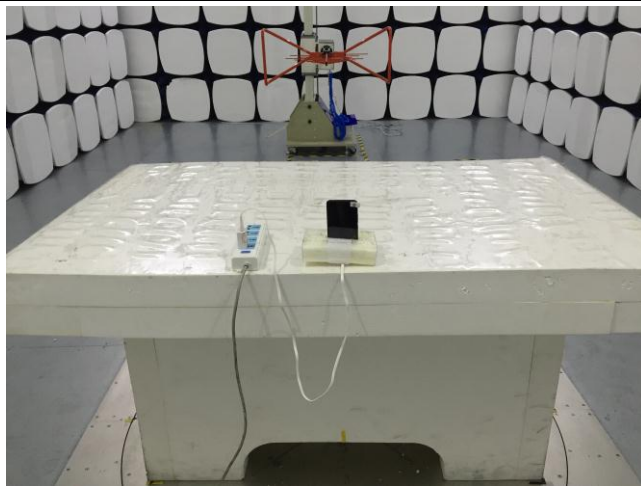
Radiated Spurious Emissions Test Setup Below 1GHz
