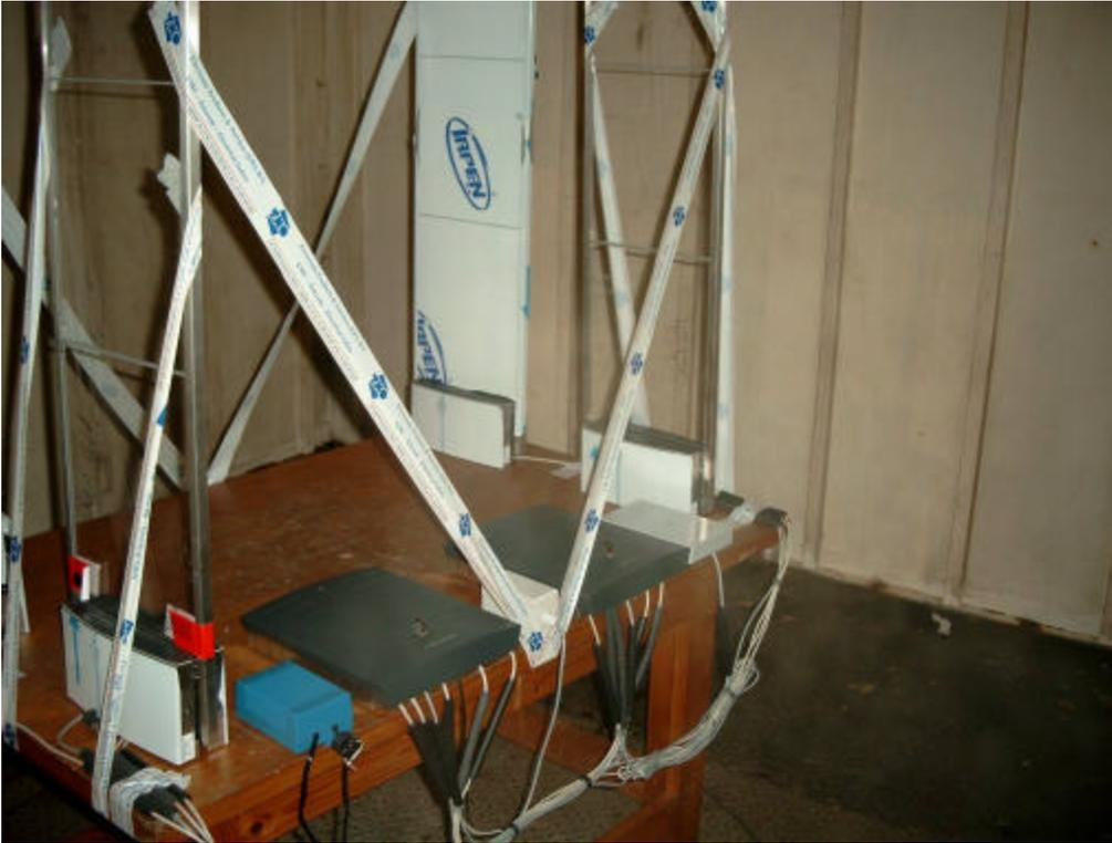
**1.5 Radiated emission test setup Configuration III (front).**
