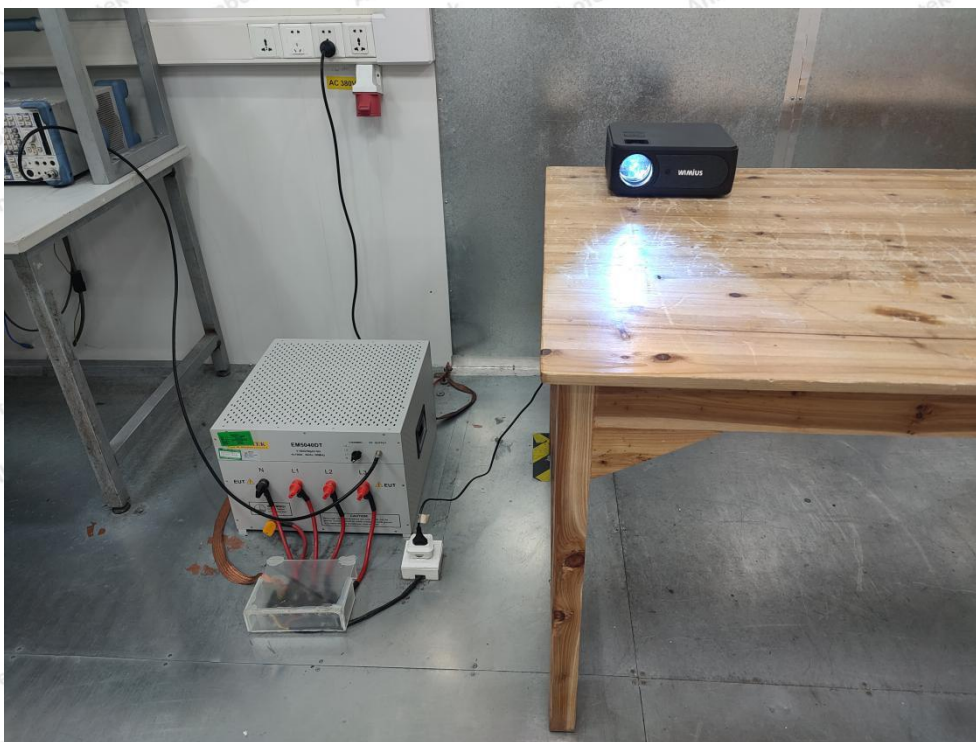
Photo of Conducted Emission Measurement
