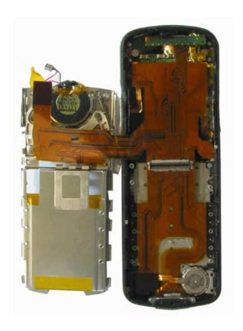
Exhibit 6: Back internal view showing interconnecting printed flexy circuit and peripherals.
