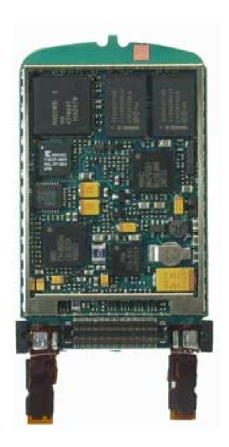
Exhibit 5: Bottom View of Printed Wire Board with screaning can removed to show baseband circuitry.
