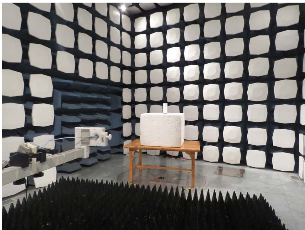
Picture 1 Radiated Emission Test Setup
