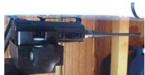
Body SAR Test Setup with 1.0cm Belt-Clip
