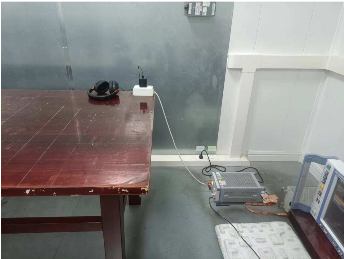
Photograph 3: Set-up photo for Conducted Emission
