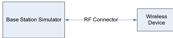
Figure 9-2 Power Measurement Setup
