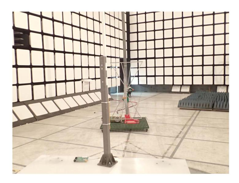
Radiated Emissions @ 3 m, Orthogonal Position 2 EUT with 15.1 dBi Yagi Antenna and 0.65 dB Assembly Cable Loss
