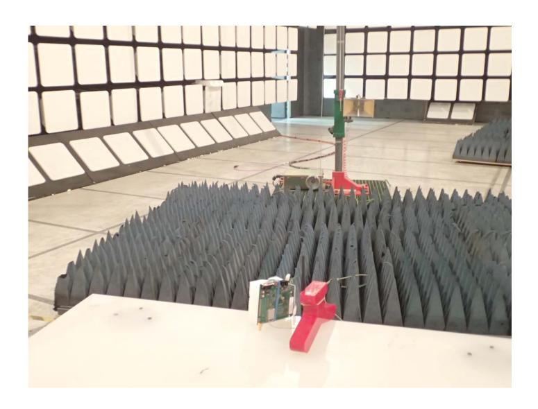
Radiated Emissions @ 3 m EUT with 3.3 dBi Monopole (Integrated Whip) Antenna and 0.44 dB Assembly Cable Loss
