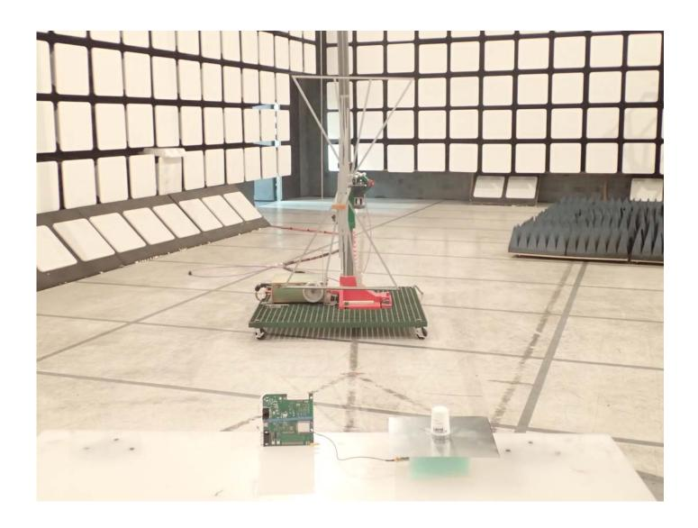
Radiated Emissions @ 3 m EUT with 2.1 dBi Dipole Antenna and 0.36 dB Assembly Cable Loss
