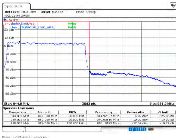
n26(824-849) SCS=15kHz DFT_QPSK BW=5MHz HighChannel=169300 RB=25@0
