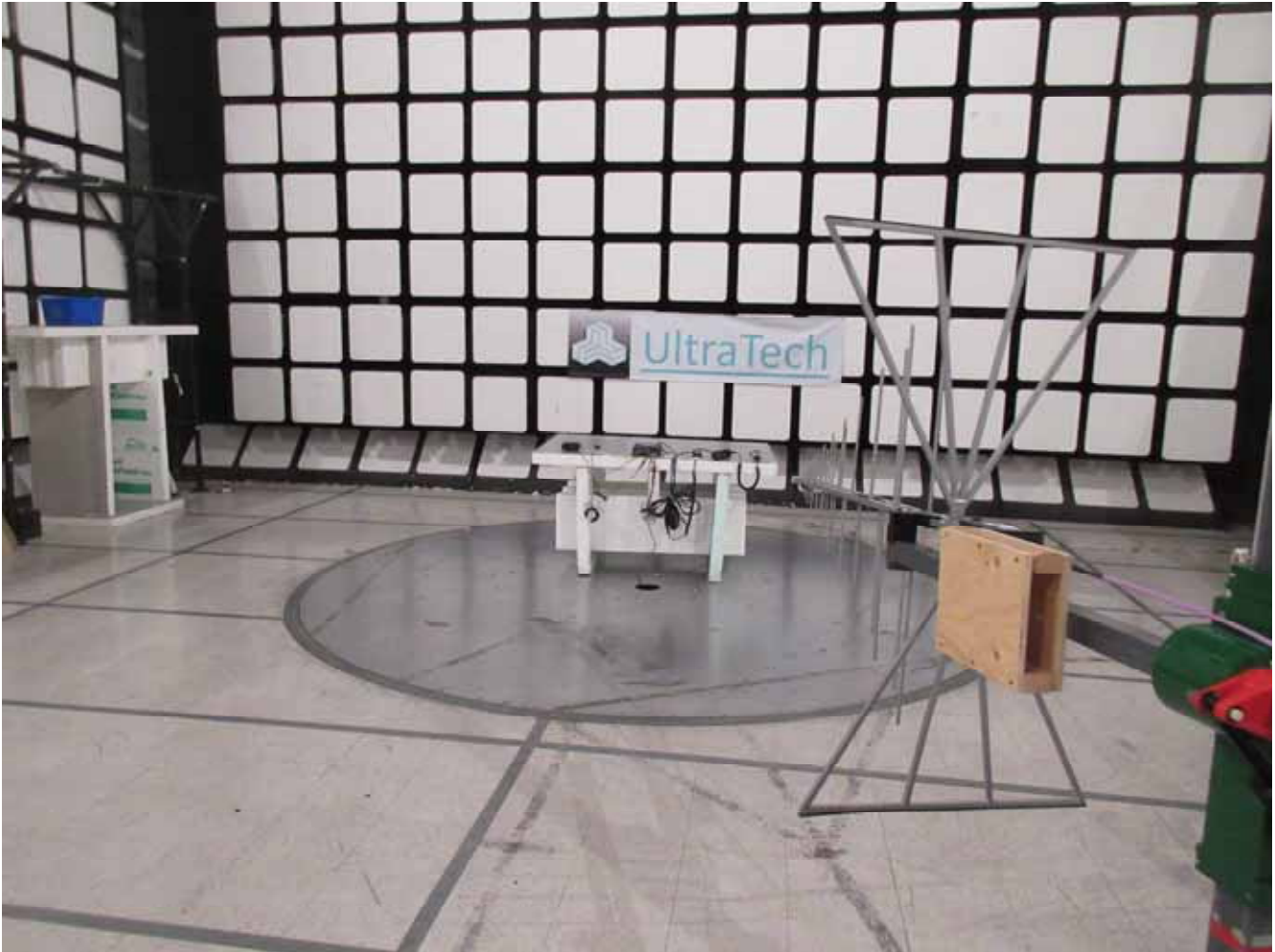
Tx Radiated Emission Test Setup
