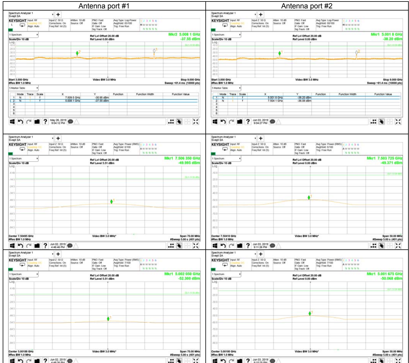
Plot 7.4.13 Spurious emission measurements in 3000 - 9000 MHz range at low carrier frequency
