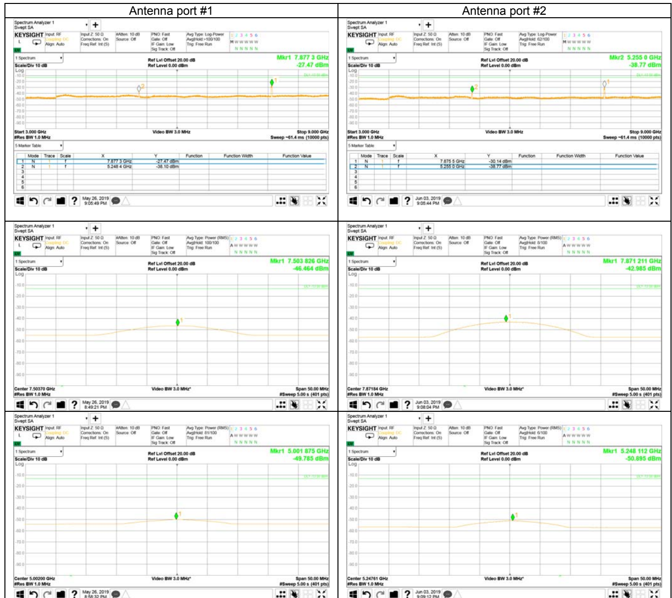
Plot 7.4.14 Spurious emission measurements in 3000 - 9000 MHz at mid carrier frequency
