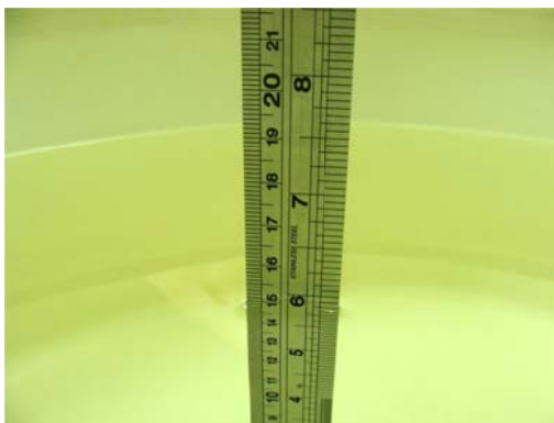
Fig 6.1 Photo of Liquid Height for Body SAR
