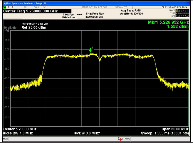
IEEE 802.11ac_Channel 46_40MHz_Antenna 0
