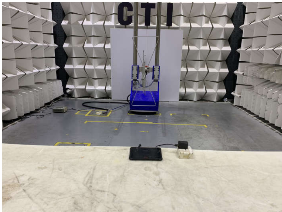
Radiated spurious emission Test Setup-3(Below 1GHz)
