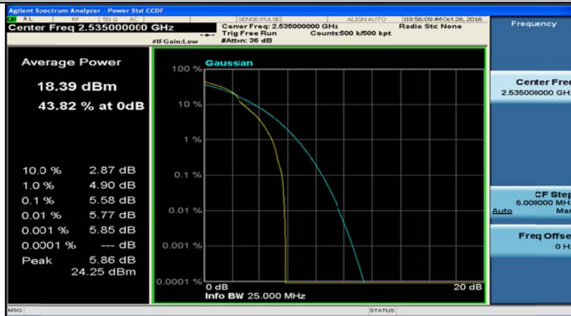
(Channel Bandwidth: 5 MHz)_MCH_16QAM_12RB#0
