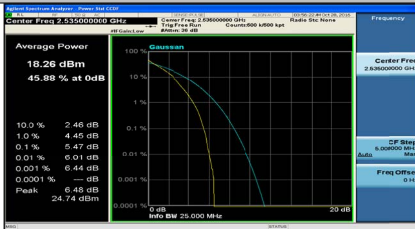
(Channel Bandwidth: 5 MHz)_MCH_QPSK_12RB#6
