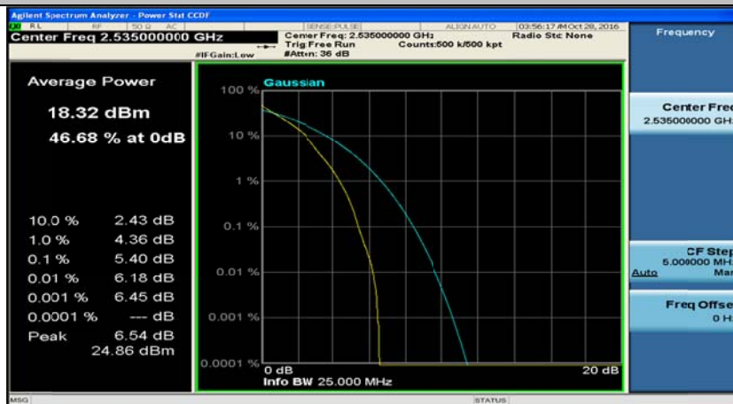
(Channel Bandwidth: 5 MHz)_MCH_QPSK_12RB#6
