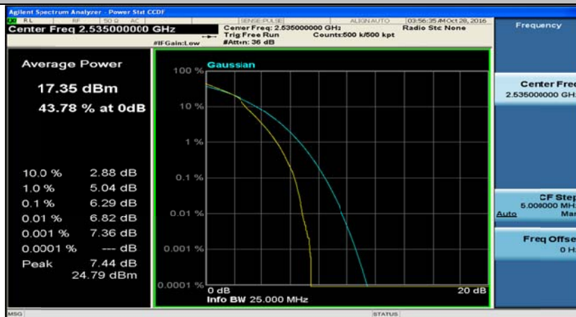
(Channel Bandwidth: 5 MHz)_MCH_16QAM_12RB#6
