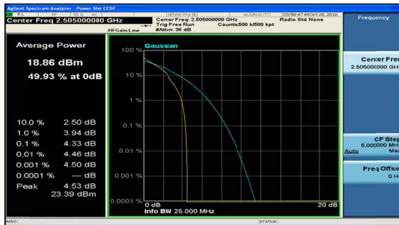
Channel Bandwidth: 10 MHz_LCH_QPSK_1RB#49
