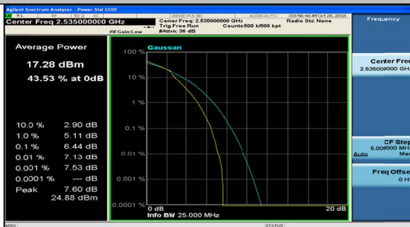
(Channel Bandwidth: 5 MHz)_MCH_16QAM_12RB#6
