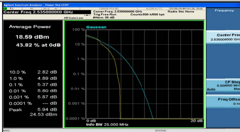
(Channel Bandwidth: 5 MHz)_MCH_16QAM_1RB#12
