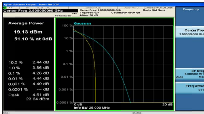
Channel Bandwidth: 10 MHz_LCH_QPSK_1RB#49
