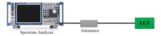
A short RF cable with low cable loss connected to the EUT antenna port, which was provided by manufacturer. The cable loss of this RF cable was offset into the setting of test equipment, which was provided by manufacturer **\( \Delta \)**.
