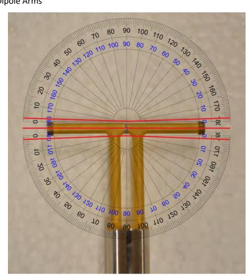
• The center red line indicates that the arms of the dipole fall within  $\pm 2^{\circ}$
