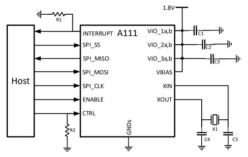
Figure 7.3. Recommended integration of the A111 radar sensor.
