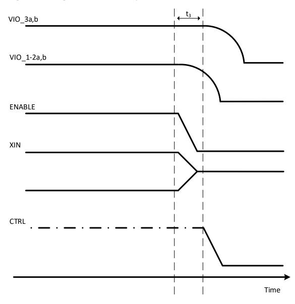
Figure 7.5. The power down sequence
