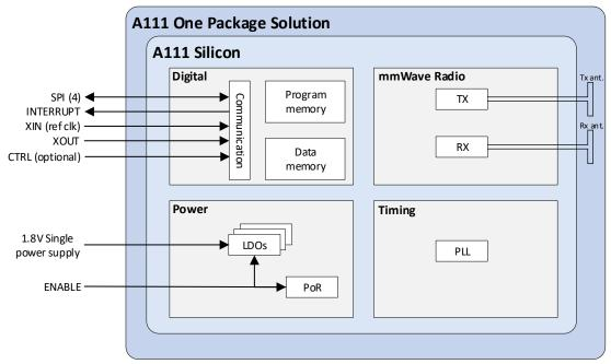
Figure 2.1. The A111 functional block diagram.
