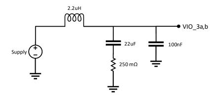
Figure 8.2: Low cost LC supply filter
