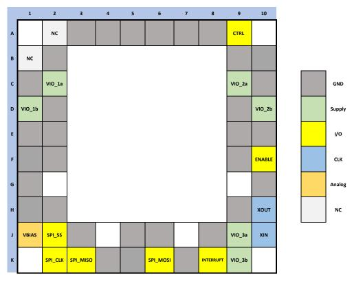
Figure 3.1. Pin configuration of the A111 sensor, top view.
