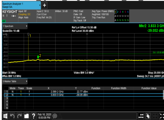
N41(10M)_DFT-s- OFDM QPSK Edge 1RB Left Mid CH
